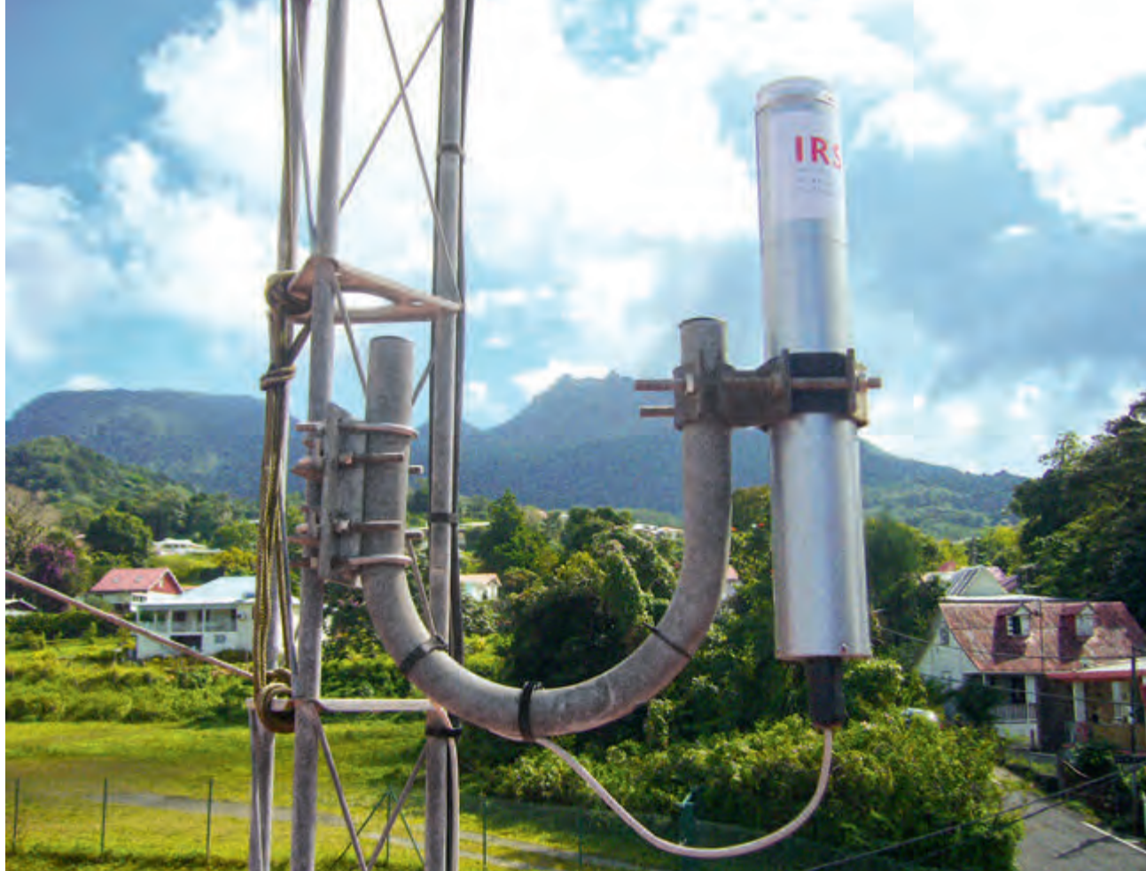
•— The deployment of new Teleray probes began in overseas France. Illustrated above is the beacon installed in Saint-Claude in Guadeloupe to monitor atmospheric gamma radioactivity.
