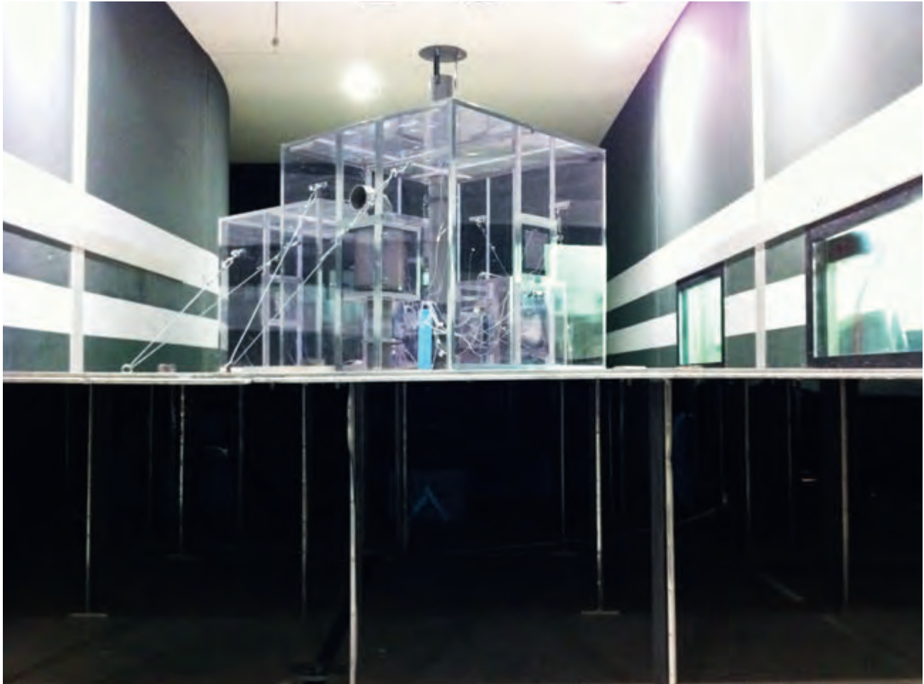
•• Many wind tunnel tests were performed on a mockup of a building representing reference facilities equipped with a ventilation network. The purpose of these tests was to measure leak rates.
