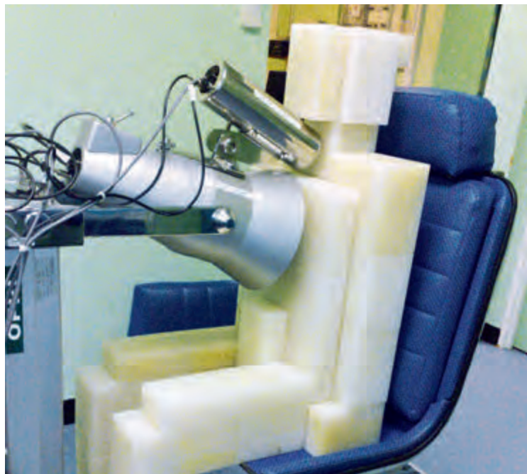
• IGOR, the anthropomorphic phantom used for testing whole body counters used at EDF facilities.
