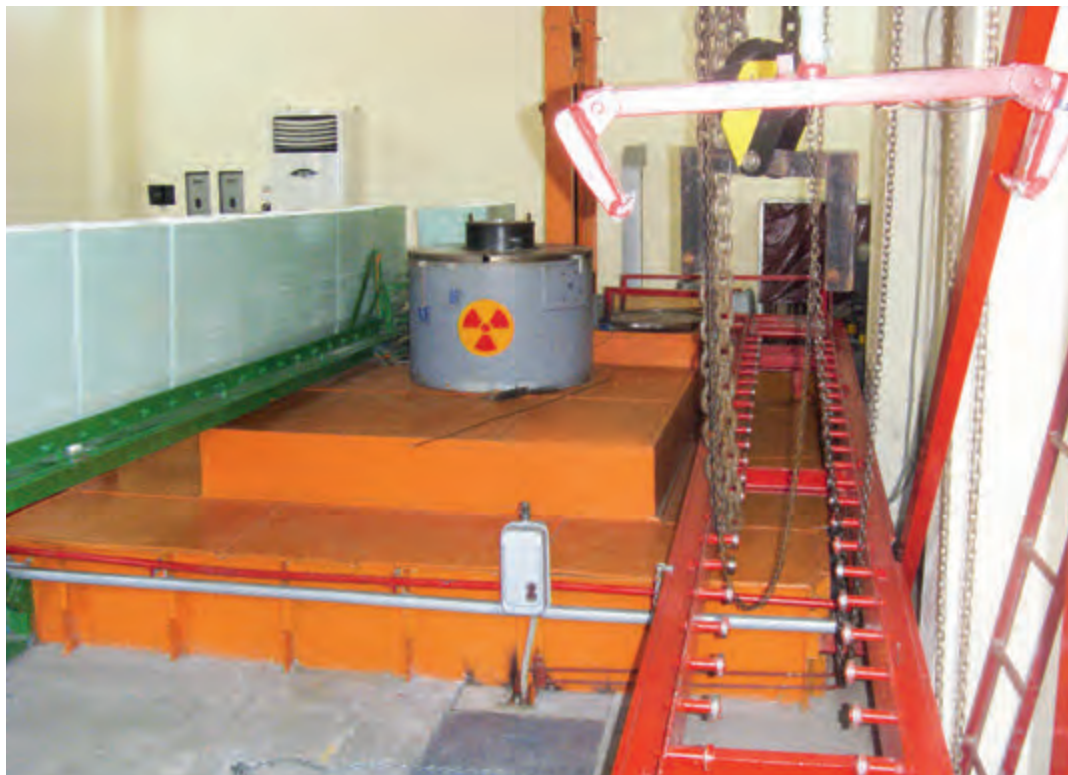
•— The cobalt source storage container at the sterilization facility was the cause of the accident in Bulgaria.
