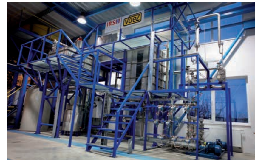
General view of the VIKTORIA loop used to conduct experiments under conditions representative of those likely to be encountered in different types of nuclear reactor during a loss-of-coolant accident.
