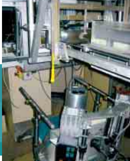
Measurement with a tissue equivalent proportional counter for the CPO proton beam line.
