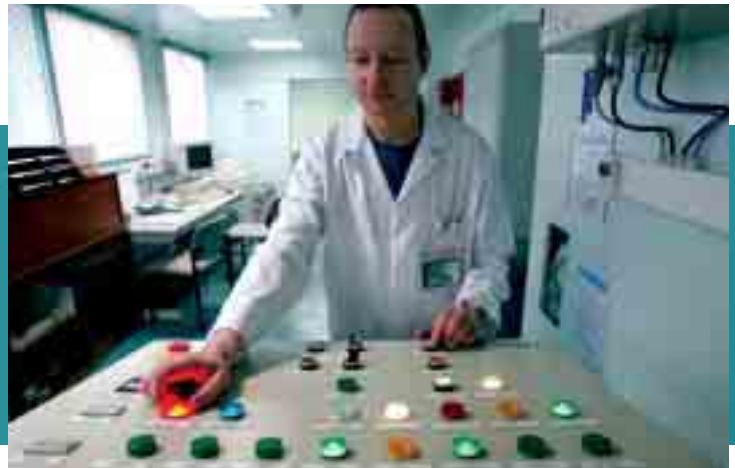
Control panel of the irradiation room for radiobiological studies or high-level dosimetry.
