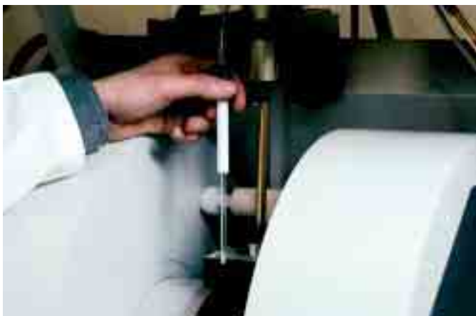
Irradiation and contamination accidents - Placing a sample for measurement by EPR spectrometry.
