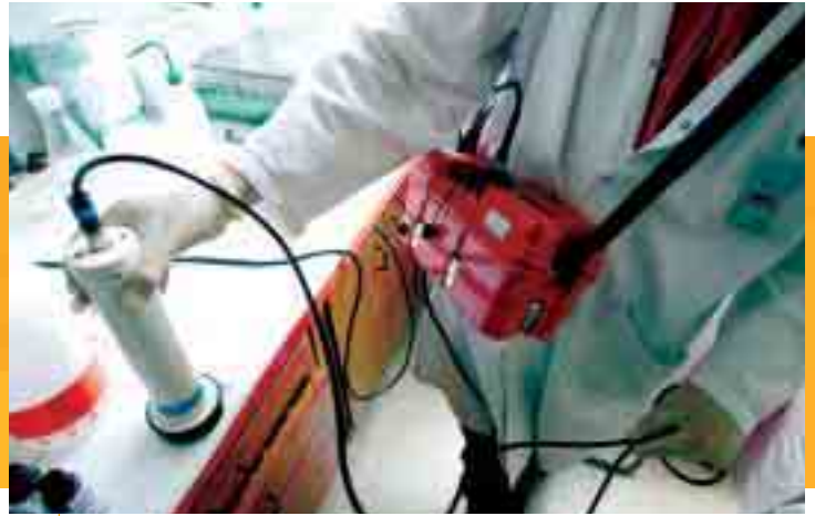
Active sample laboratory: radiological check to verify the non-contamination of a fume chamber laboratory.
