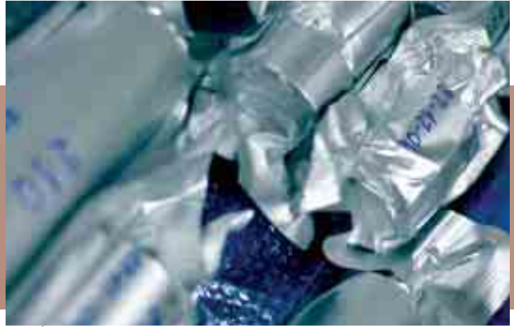
Vacuum packing of clay samples taken at Tournemire for chemical analysis in the laboratory.
