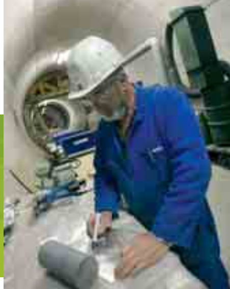
Packaging and reference marking of clay core sample taken at Tournemire (Aveyron).
