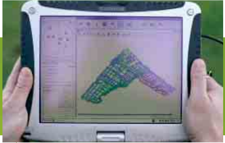
Map of the gamma dose rate in real time with respect to geographic location.
