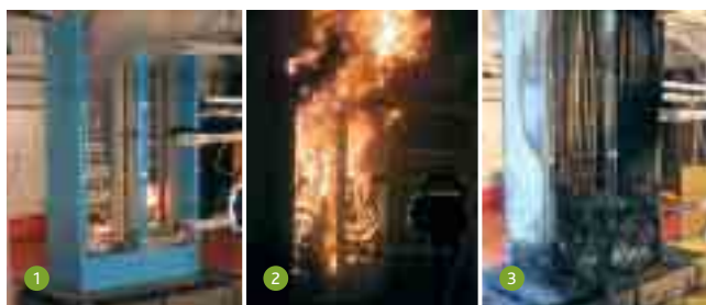
Test aimed at ascertaining electrical cabinet combustion modes. 1- Ignition phase. 2- Fully developed fire. 3- Post-experimental phase.
