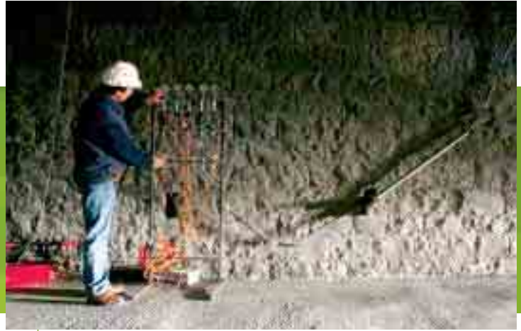
Instrumentation used to monitor changes in the rock after drilling.
