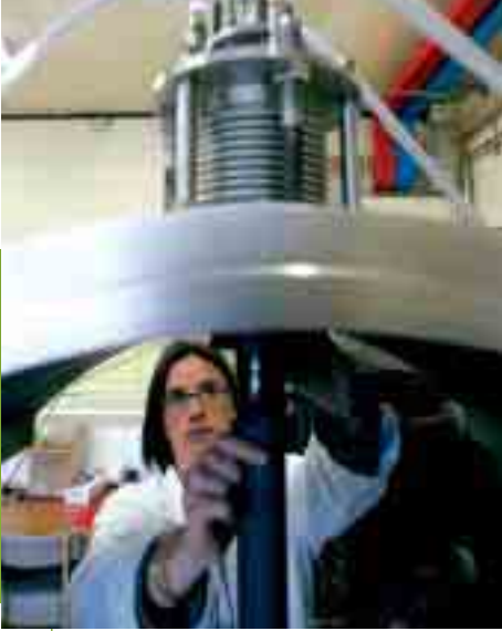
Fitting the test section in the Intermezzo furnace.
