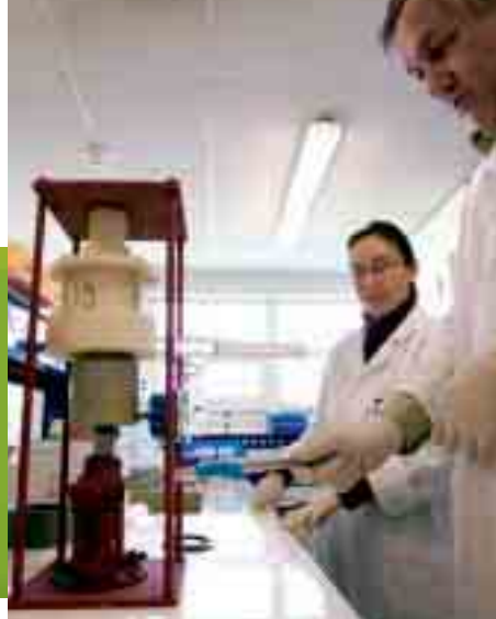
Sediment press used to extract interstitial water for analysis.
