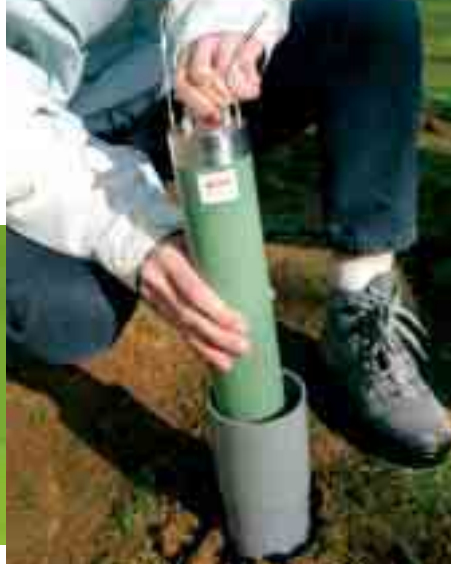
Probe measuring radon concentration in the ground.
