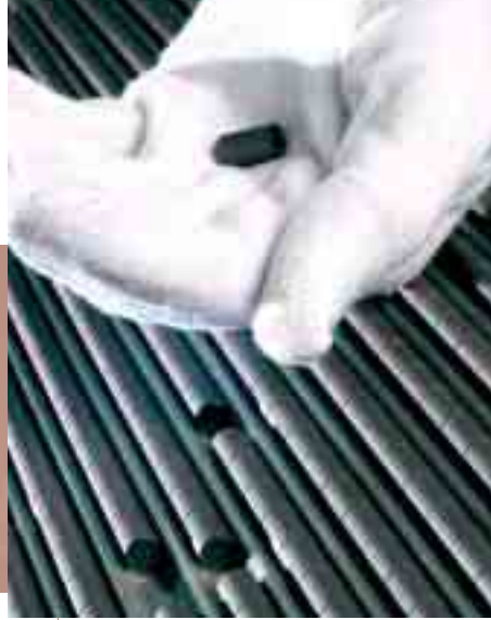
UO 2 pellet constituting the fuel for a PWR.
