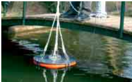
A portable Telehydro probe has been developed to take measurements at precise points along water courses.
