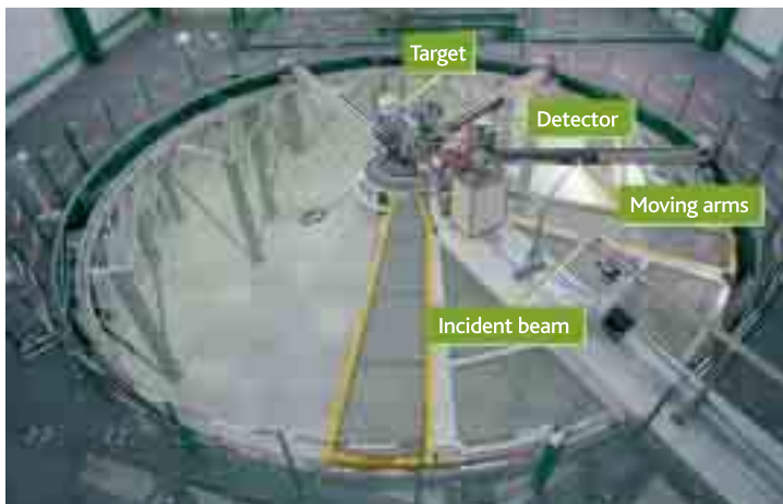
Test hall for the AMANDE installation.
