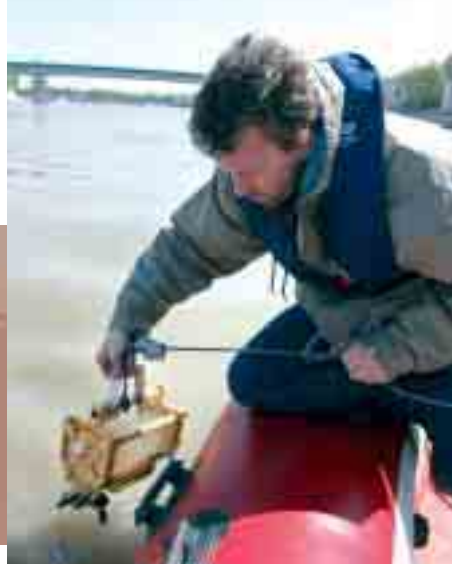
During flood periods, the Institute takes greater numbers of samples of river sediments which may contain the main part of annual radionuclide flows.
