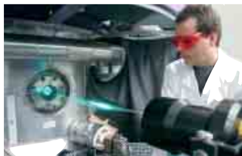
Apparatus for laser measurements using a new technique: rainbow refractometry.
