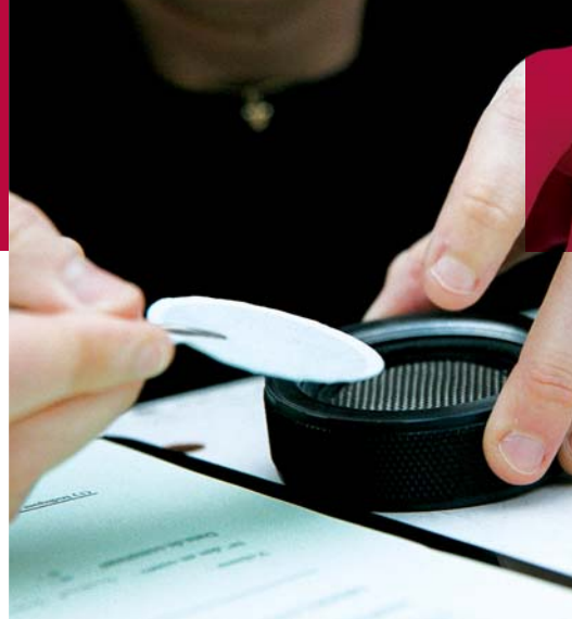
Filter used to collect aerosols.
