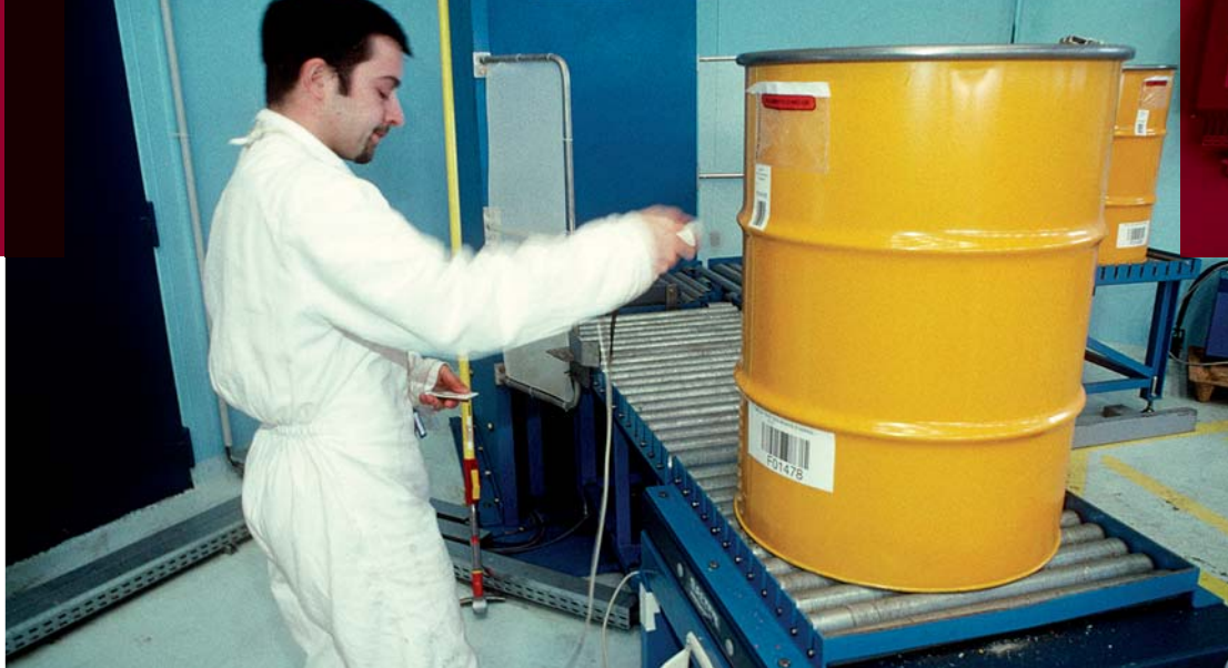
Nuclear material measurement in a drum.
