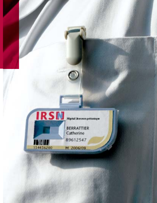
Prototype RPL dosimeter.
