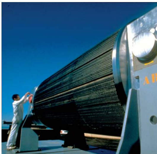
Irradiated fuel shipment container.
