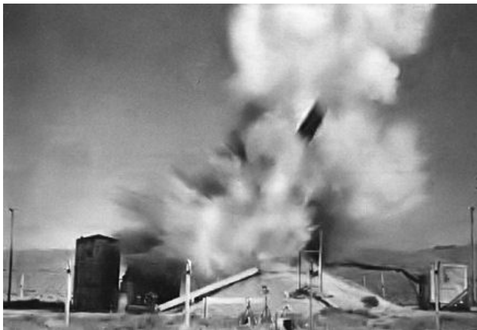
Figure 4. Photography taken during the "destructive" test on the BORAX-1 reactor.
