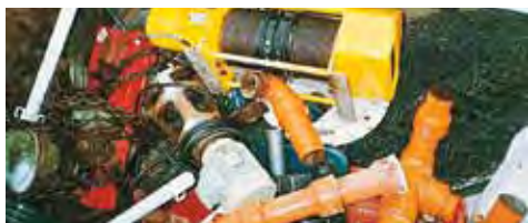
VLLW waste includes rubble, scrap and pipes mainly from dismantled nuclear facilities.
