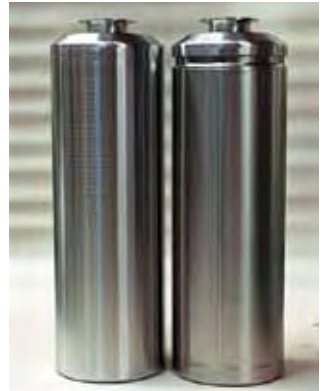
Containers of waste, vitrified on the left and compacted on the right.
