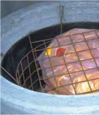
Solid waste in its concrete drums, before covering with cement.
