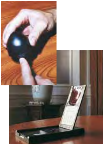
Examples of dosimeters used by the IRSN for measuring radon levels in buildings.
