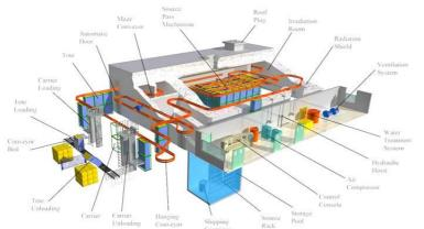
Standard diagram of an irradiation facility
