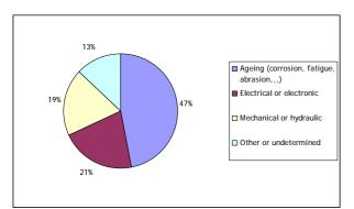
Breakdown of causes of equipment failures
