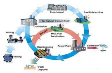
The operations to prepare and manufacture the nuclear fuel intended for use in nuclear reactors ("front end") and to reprocess the spent fuel after use ("back end") form the nuclear fuel cycle.<sup>1</sup>
