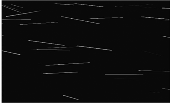
Fig. 4 High-speed camera visualization of incandescent particle trails in the measuring section
