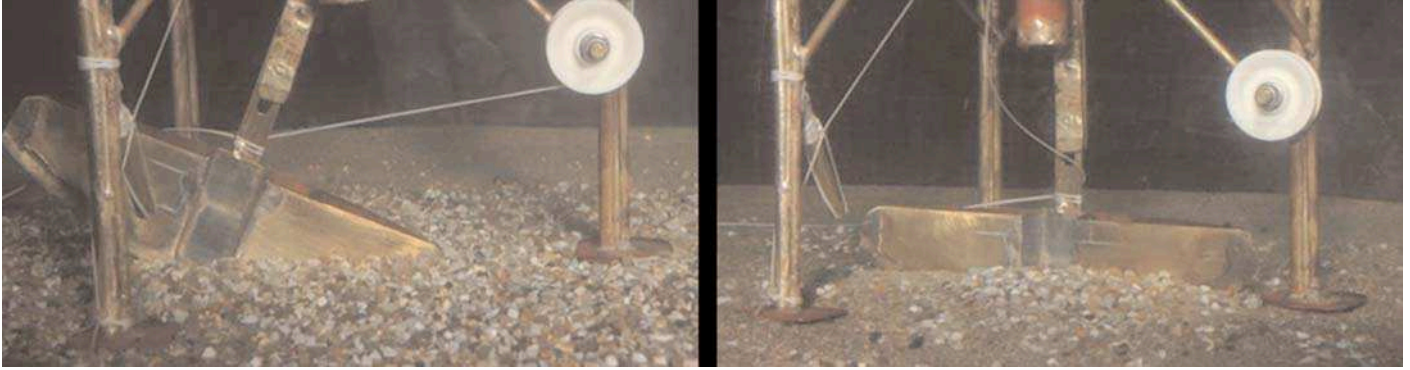
Fig. 5. 1/10 scale model of the walking beam deployed in a flume.
