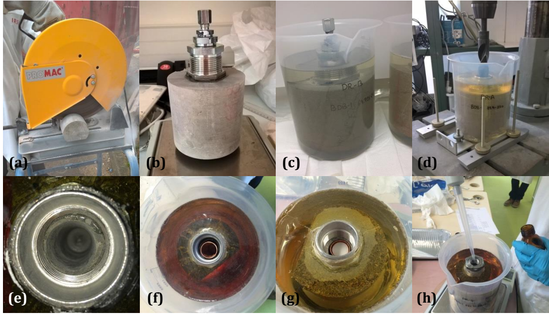
Figure 2.13: Preparation steps of radial diffusion experiments (a) Core sawing using a circular saw (b) Plug fixation on the core (c) Resin-coated core sample in a beaker (d) Reservoir drilling (e) Empty reservoir (f) Insertion of the copper tube (g) Insertion of the PTFE rod (h) Pouring of the resaturating solution
