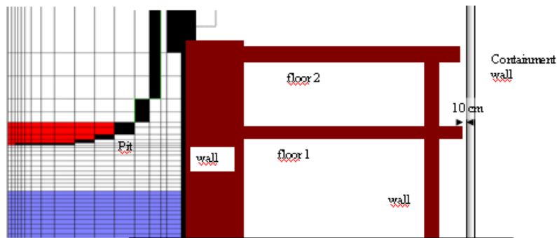
Fig. 45 : Representation of geometry for French PWR 900 MWe reactor analysis
