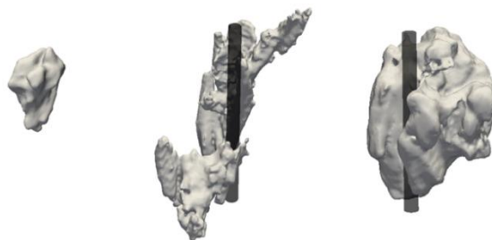
Figure 5: Selected bubbles in the single tube set-up with a guillotine break. The bubble diameters vary between 50 and 140 mm
