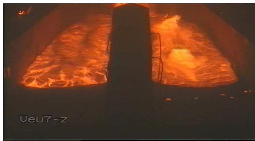
Figure 6.3-1: Spreading of prototypical corium over ceramic ridges (left) and concrete ridges (right) [VULCANO test VE-U7]
