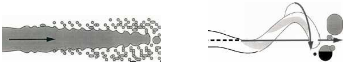
Figure 4.3-3: Instability/fragmentation via atomisation (left) and on a larger scale (right)
