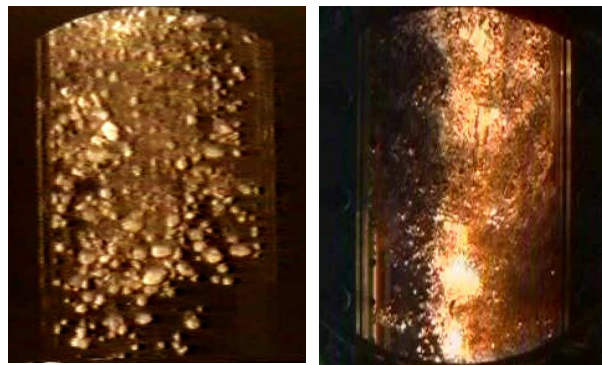
Figure 4.3-2: At left, alumina/water premixture (KROTOS-57). At right, corium/water premixture (KROTOS-58). Video camera, 24 frames/s. 10x20 cm window. Taken from [4.3_1].
