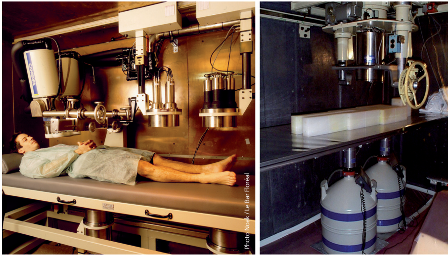
Figure 20. In vivo measurement with 4 germanium detectors (left) and efficiency calibration using the IGOR phantom (right) at IRSN, Le Vésinet.
