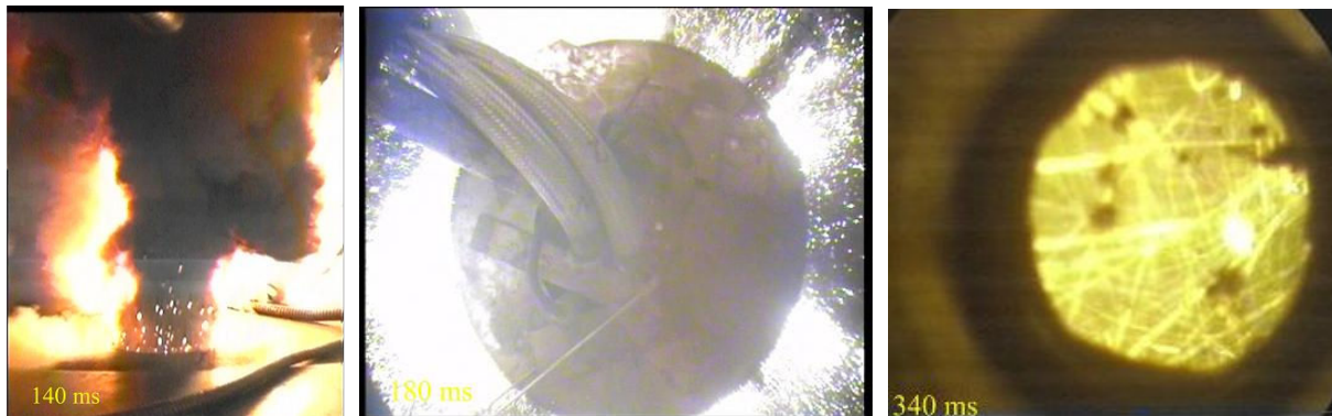
Figure 9: Photos from camera recording during test DISCO-L1. Left : camera looking inside the containment, just above the compartment, middle : camera looking downward above the RPV, right : endoscope looking in the compartment
