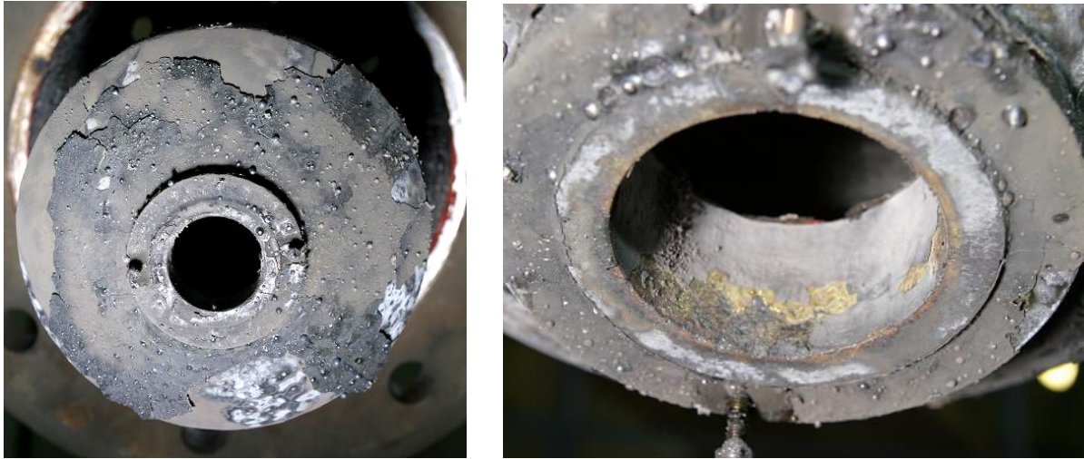
Figure 8: Left : View of the lower head vessel with homogeneous crust from below; Right : View of the breach after the test with some brass around it
