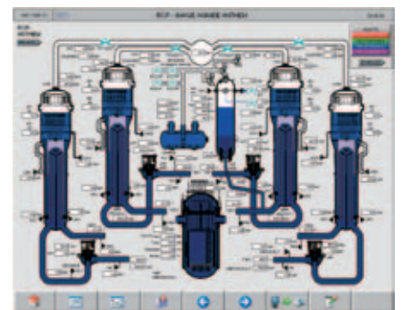
EPR reactor under normal operation. Liquid water appears dark blue, whereas steam appears in white.
