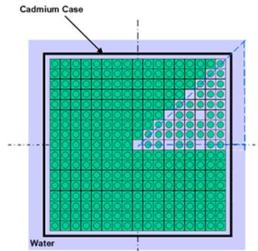
Figure 2. Multi-cell geometry for APOLLO2 calculation
