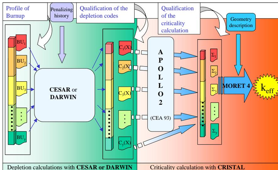
Figure 5. Process to take Burnup Credit into account in a criticality calculation with CRISTAL V1
