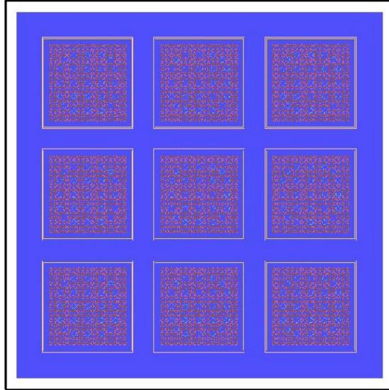
Figure 4. TRIPOLI-4 horizontal cut of the 3D representation of a storage of spent fuel assemblies
