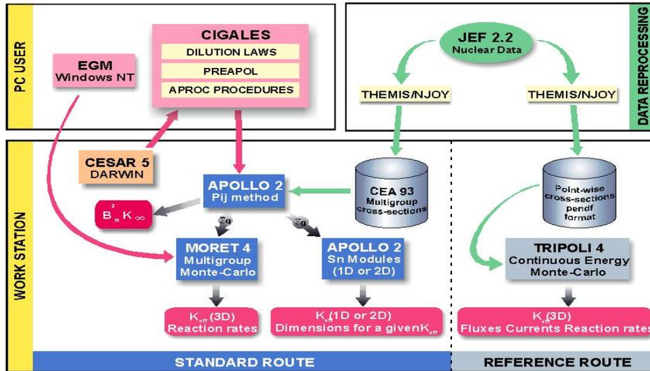
Figure 1. Functional architecture of the CRISTAL V1 package.
