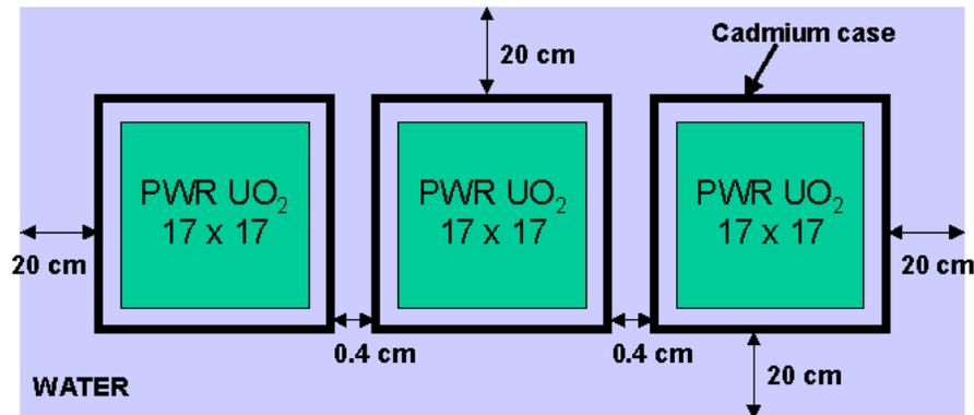
Figure 3. Horizontal cross-section of the 2D representation of a storage of spent fuel assemblies
