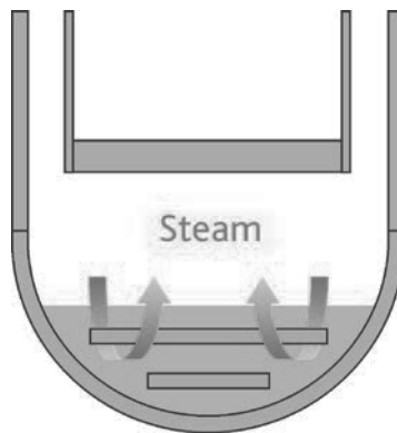
Figure 5.3. Schematic diagram of corium configuration after the lower head has dried out: a debris bed (which is more or less porous, depending on the degree of fragmentation of the corium) around steel structures, with steam circulating through natural convection.
