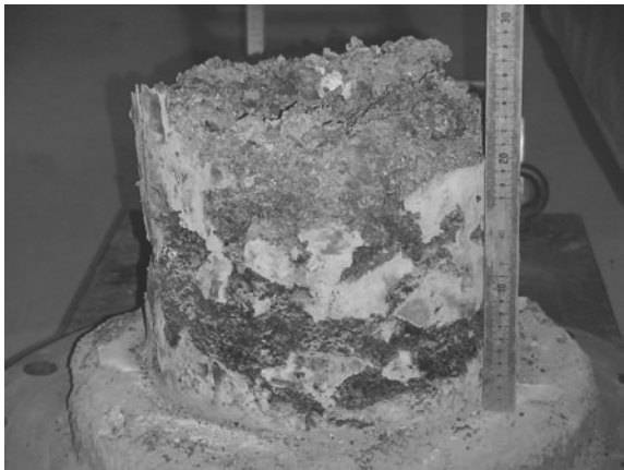
Figure 5.49. Appearance of the resolidified lump of corium at the end of the SSWICS-11 test, performed with gas injection into the corium, see [32]; reproduced by permission of OECD.
