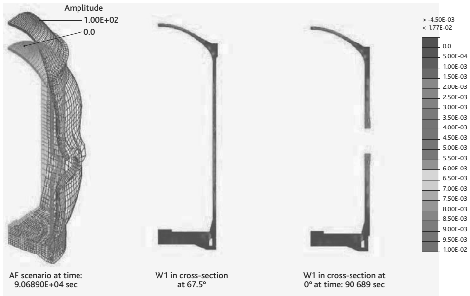
Figure 6.6. Containment strain amplified 100 times and concrete cracks, in the equipment hatch axis and the main body, at the pressure peak of the AF scenario (time P3).
