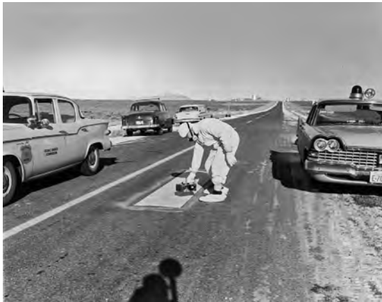
Figure 8.2. Measurement of ground contamination near Reactor SL-1. @ INL.
