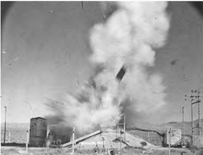
Figure 8.3. Top, diagram of the BORAX-1 reactor. © All rights reserved. Bottom, photograph taken during the final destructive testing of the BORAX-1 reactor. © Argonne National Laboratory ( creative commons ).
