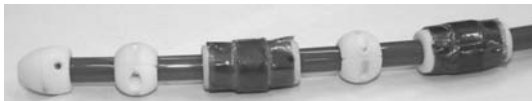
Figure 10.10 Prototype of a flexible eddy current sensor for examining SG tube bends. © DR.
