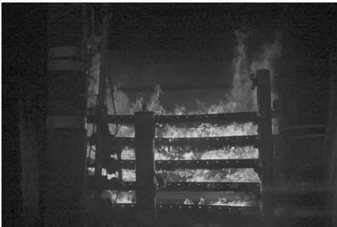
Figure 7.5 An experiment involving a fire in a set of cableways, one on top of the other. © Florent-Frédéric Vigroux/IRSN.
