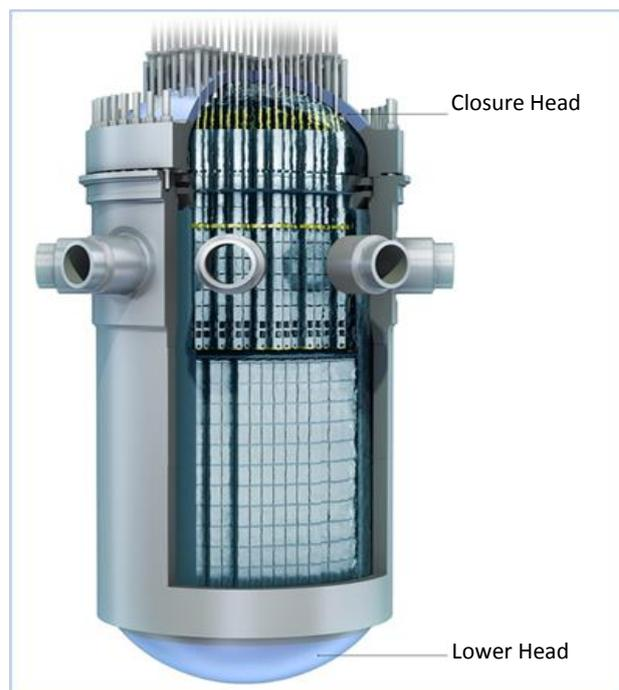
Diagram of the EPR reactor pressure vessel
