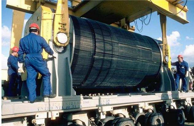
Figure 19: TN 12/2 package during loading on a lorry
