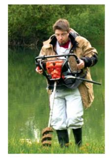
Mechanical auger for soil sampling.
