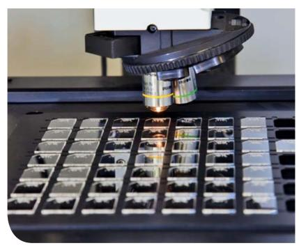
Reading neutron dosimeters.
