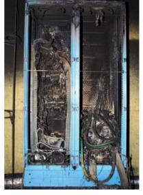
Electrical cabinet after a PICSEL EP test at the DIVA facility.
