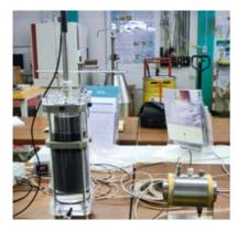
Experimental set-up used to study gas production by irradiation.
