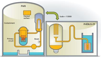
PHEBUS FP facility - a 1:5,000 scale replica of a PWR.
