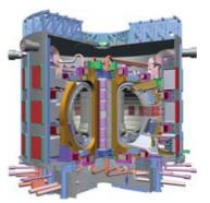
ITER: cross-sectional view of toroidal magnet.
