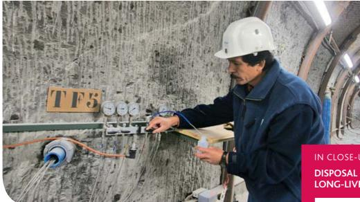
Taking water samples for geochemical analysis at the front of a chemically inert system, isolating a transmissive fracture in the Tournemire experimental station.
