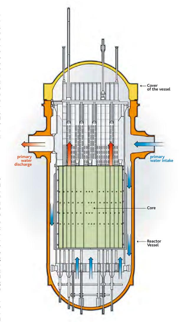
■ Cross-section of the vessel of a 900 MWe pressurized water reactor.
