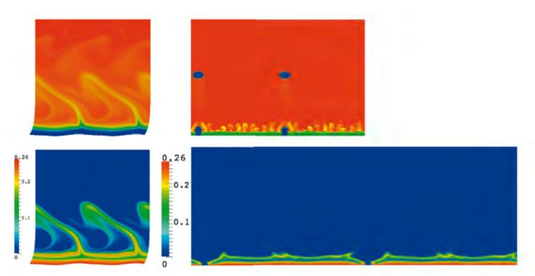
■ Display of the interface between corium and siliceous concrete with (right) and without (left) gas release. Density deviation (top) and solid fraction deviation (bottom).
