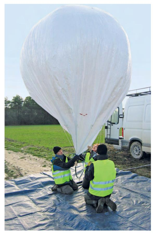
Preparing IRSN's captive balloon for high-altitude tracer gas measurements.
