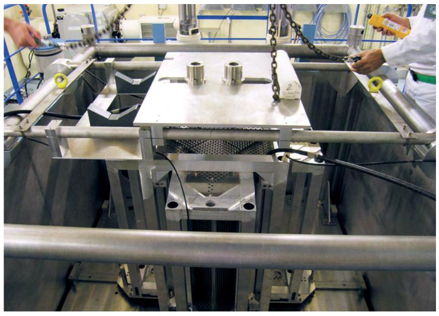
■ Installing the "fine" test device with its 5 mm copper shield in equipment test tank B of the criticality facility at the CEA Valduc site.
