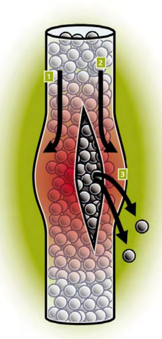
■ Schematic illustration of the fuel relocation phenomenon and fuel ejection in the event of cladding failure. 1. Fuel cladding. 2. Fuel fragments (shown as spheres). 3. Clad ballooning and cracking induced by fission gas pressure in the fuel.
