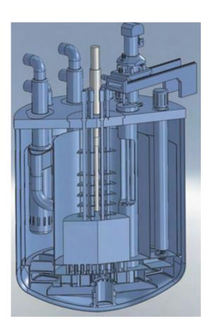
■ Schematic illustration of the Astrid reactor.
