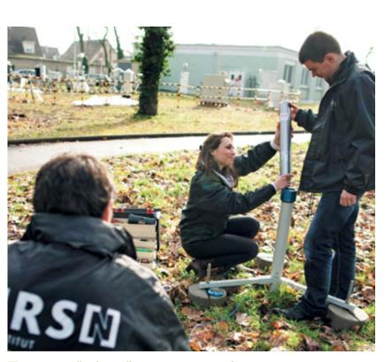
■ Testing a "Teleray" new-generation beacon.
