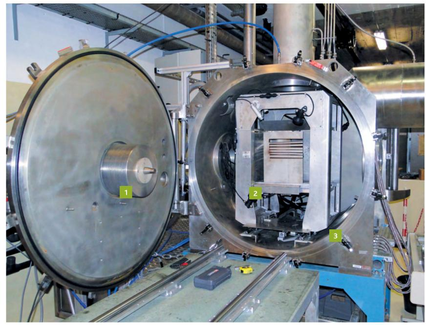
■ The work carried out in cooperation with the CEA's joining technology laboratory (LTA) in Saclay, near Paris, involved the use of the continuous wave 8 kW YAG laser at the DELIA facility, for underwater and air laser cutting facility. 1. Laser cutting head 2. Steel plate 3. Underwater cell.
