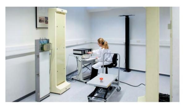
■ IRSN tests the performance of radioactive material detection barriers.
