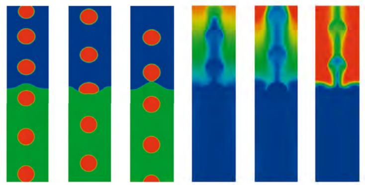
■ Change in an interface in the corium between an oxide layer and a metal layer with gas bubbles released by the concrete passing through it. Density deviation on the left and temperature fields on the right used to quantity heat transfer.
