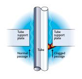
In 2005, it was reported that the passages left to allow water and steam to flow between the tubes and the tube support plates had, in some steam generators, become gradually clogged with oxide – mainly magnetite – deposits 724 Technical notices to the nuclear safety authorities (excluding defense-related activities) (690 in 2006)
