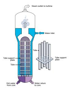
Each SG contains around 3300 inverted-Ushaped tubes that the tube support plates help to keep in place.
