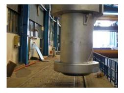
IR 800 irradiated fuel element transport package.
