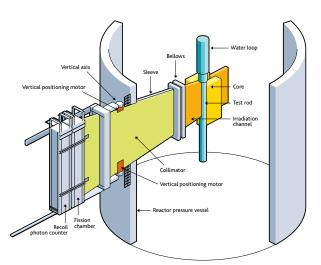
The hodoscope is used to take real-time measurements of fuel movements inside the test rod.
