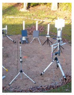
Platform used to assess ambient gamma does rate measuring instruments selected to modernize the Téléray network.
