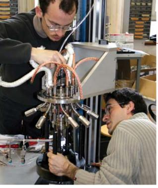
Assembly of the reactor (bottom) and furnaces (top).
