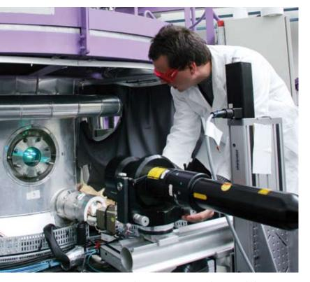
Laser velocimetry measurements in the TOSQAN facility.
