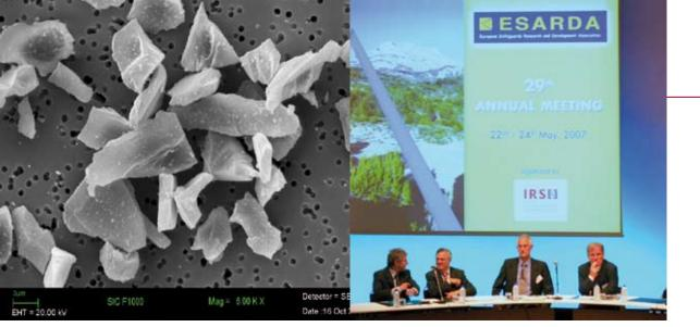
Carborundum micrography used in testing powder resuspension.
