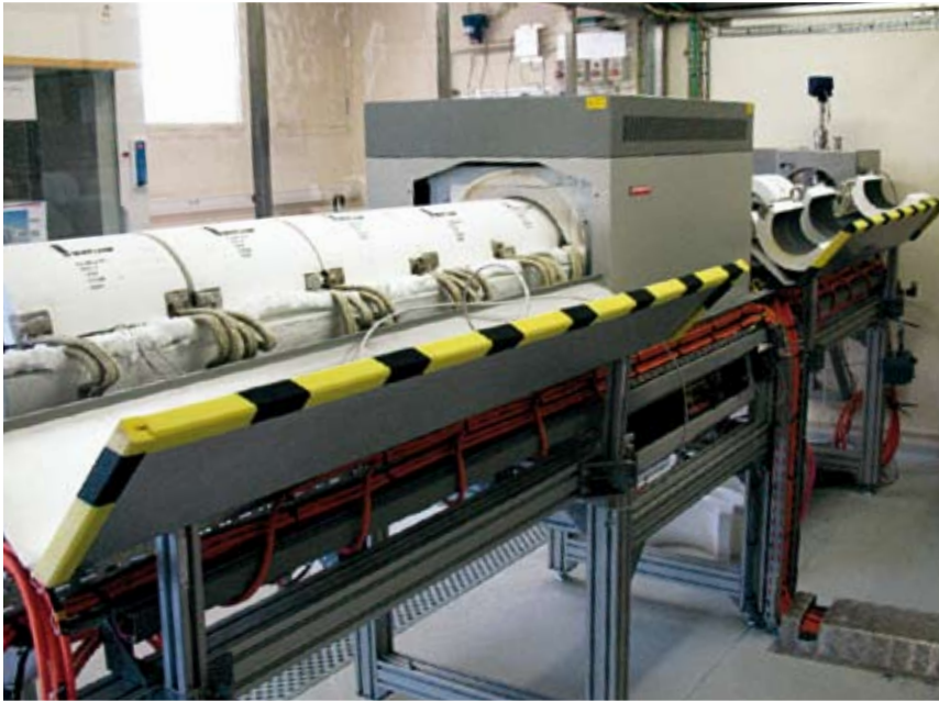
Temperature-gradient oven in the CHIP experimental facility.
