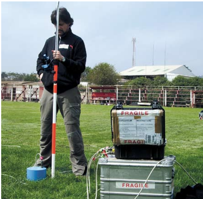
Setting up measuring equipment for characterization of the geological environment in Chili.
