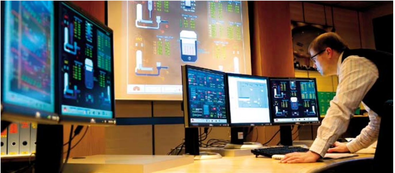
Reactor operation with the plant in service can be studied using the renovated simulator.
