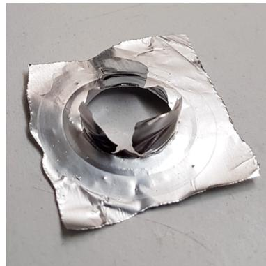
(c) Membrane of aluminum foil after rupture
