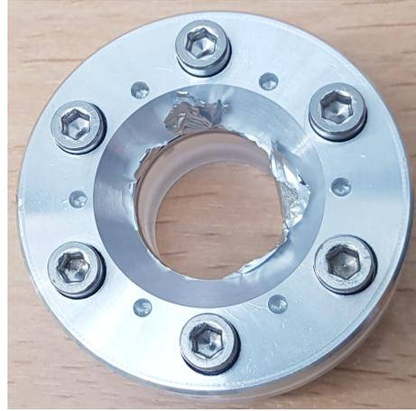
(b) Membrane of aluminum foil after rupture
