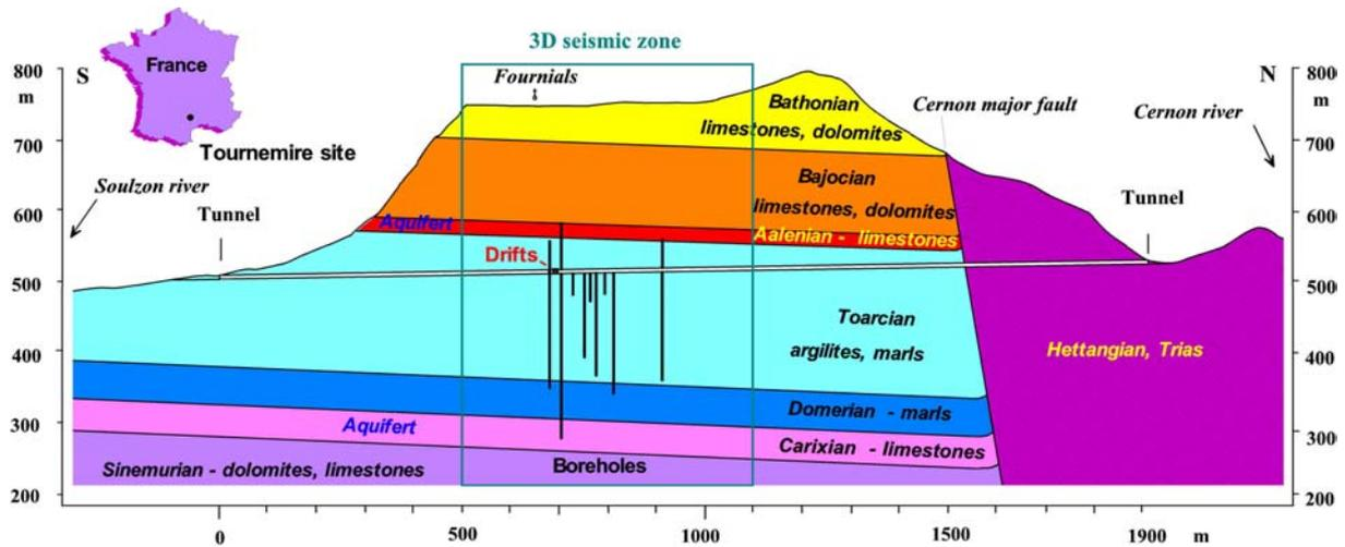
Fig. 1. Cross-geological section of the Tournemire site showing the 3D seismic zone
