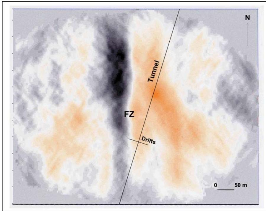
**Fig. 7.** Isochrone map in the limestone lower layer showing a roughly N-S trending fault zone (FZ).
