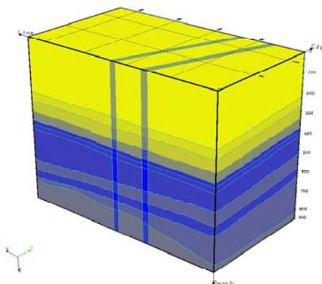
**Fig. 3.** Geological and property model with two vertical secondary fault zones used for the numerical approach (yellow – 5000-4000 m/s and bleu 3500-3000 m/s).
