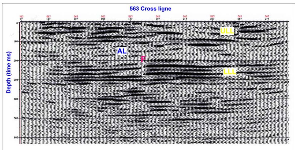
**Fig. 6.** 2D migrated section showing a break (fault) in lower limestone layer. ULL-Upper limestone layer, AL – Argillaceous layer, LLL – Lower limestone layer, F, Fault zone.
