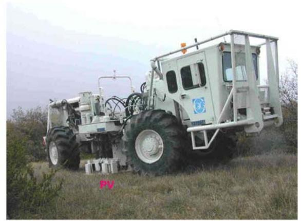
**Fig. 5.** Reception (geophones) and emission (M22 vibrator) device.
