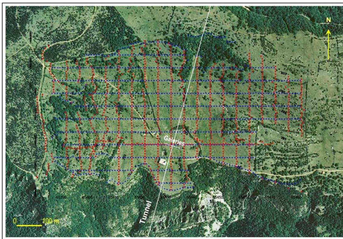
**Fig. 4.** 3D seismic field device on the Tournemire site with tunnel and drift locations (Bleu, geophones lines and red emissions lines).
