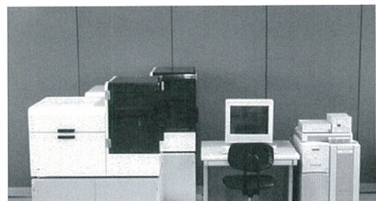
Figure 3. Exterior of automatic reader FGD-650 and server computer system
