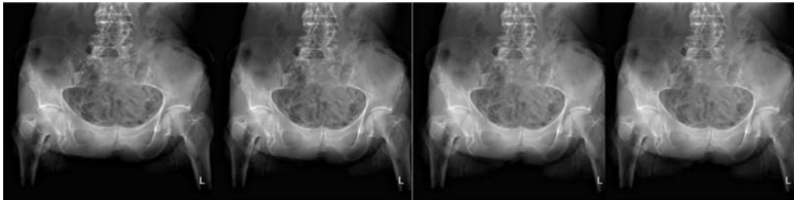
Fig. Pelvic radiographs taken at 81 kV with a Siemens Axiom Aristos FX showing the effect of additional copper filters. Exposures from left to right were taken with the following thicknesses of copper 0 mm, 0.1 mm, 0.2 mm, and 0.3 mm, and KAP values are 34 cGy cm 2 , 22 cGy cm 2 , 14 cGy cm 2 , and 11 cGy cm 2 , respectively (cadaver study- Dean Pekarovic, University Medical Centre Ljubljana, Slovenia).
