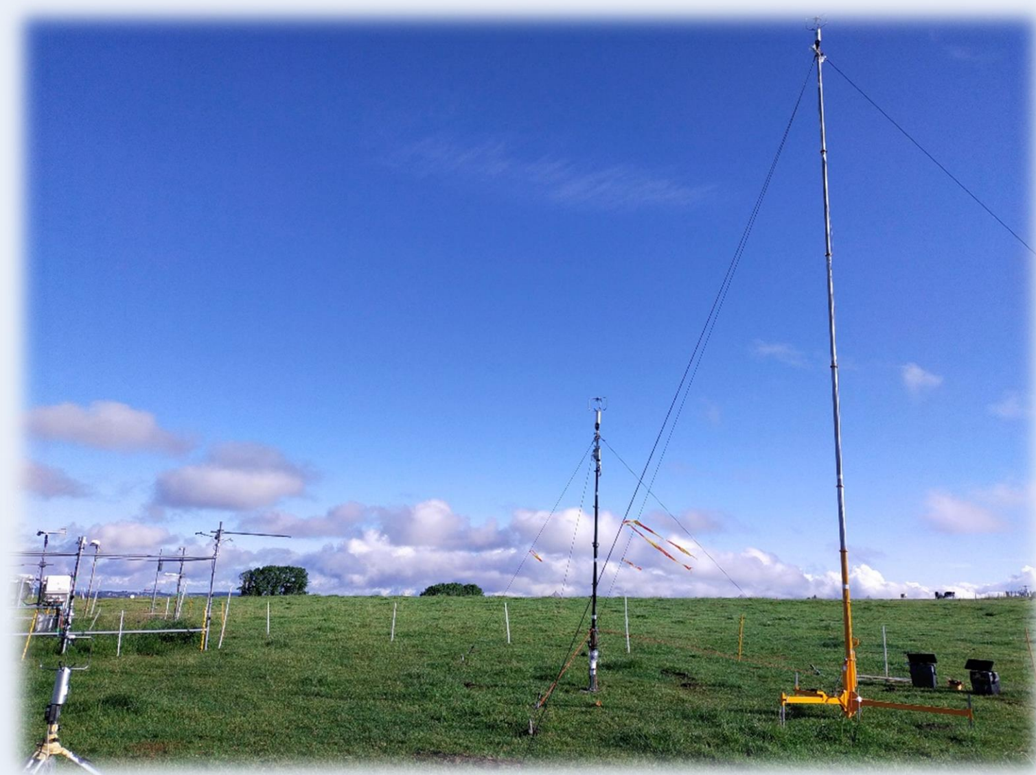
Characterization of micrometeorological conditions: ultrasonic anemometers and meteorological station
