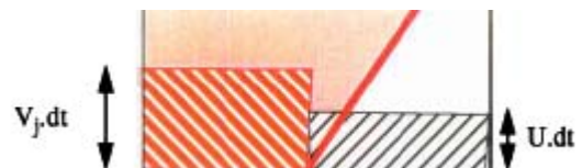
Figure 4: Convected volume with the VOF-SLIC method: red = tracked fluid.
