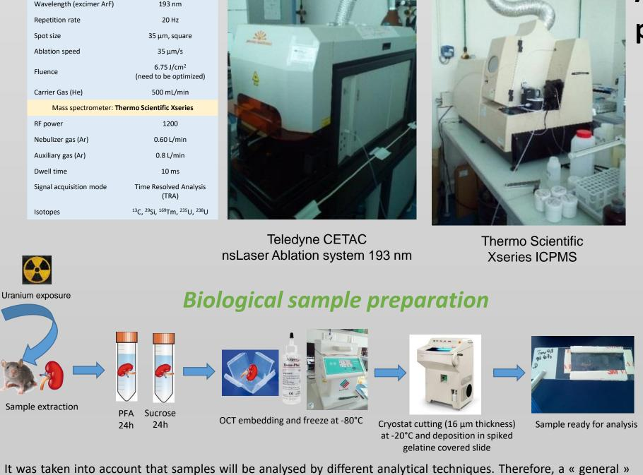
sample preparation was done in order to guarantee technical compatibility. However, the authors were aware of the fact that sample preparation might modify the initial metal distribution due to the leaching of metals from the tissue to PFA/sucrose solution<sup>9</sup>. For that purpose, both PFA and sucrose baths (after 24h in contact with kidney samples) were after analysed by ICPMS confirming that no uranium migration happened.
