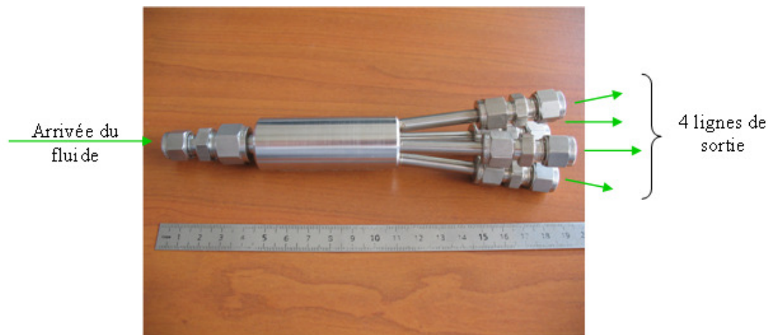
Figure 2.6: Photo du montage 'splitter'
