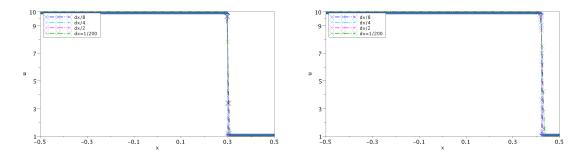
Figure B.1: Upwind Scheme for (B.4)-(B.9) (left) and (B.7)-(B.9) (right) with different mesh sizes, CFL = 1.
