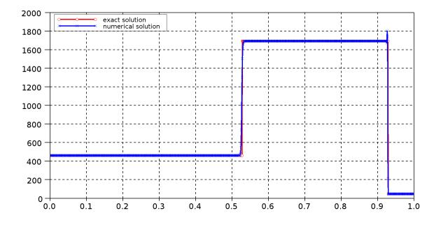
Figure 3.26: Test 5 – h = 0.001 and  $\delta t = h/5$  – Pressure at t = 0.035.
