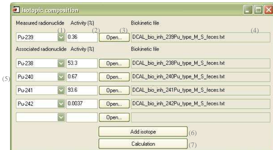
Figure 7.6: GUI to create the biokinetic file of a mixture of radionuclides in the module “Uncertainty dose calculation” of OPSCI
