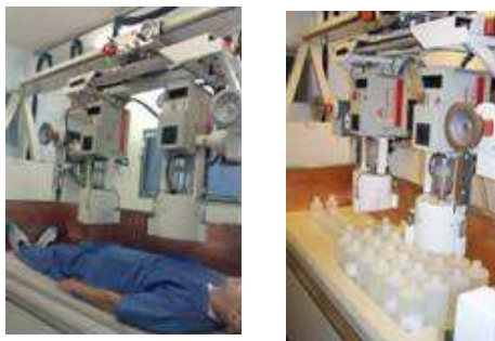
Figure 1.5: In vivo measurement and efficiency calibration using a physical (bottle) phantom in the mobile in vivo count laboratory of IRSN
