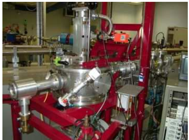
Fig. 35: AIFIRA facility. On the left, the 3.5 MV singletron; on the right the target chamber of the micrometric beamline.
