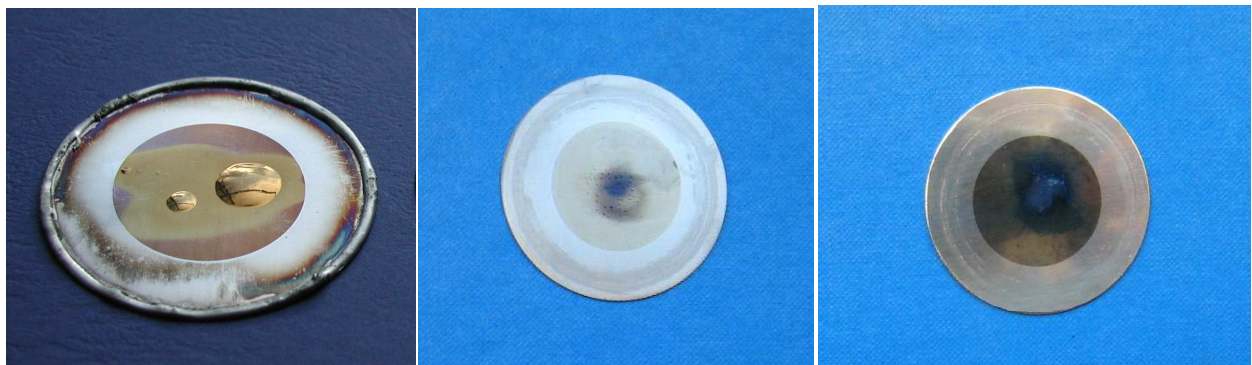
Fig. 41: Targets after irradiation at NPL: backings with bubbling as previously observed (left) and presently obtained with W (centre) and Pt backing (right) with colour change.
