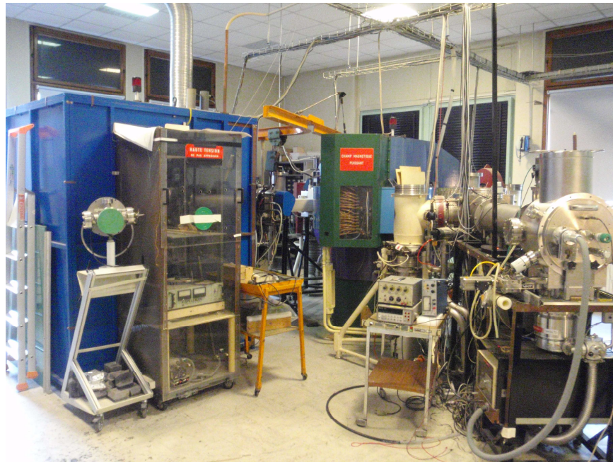
Fig. 71: SIDONIE facility. On the left, in blue, the ion source; in the middle the analysis magnet; on the right, the target chamber.
