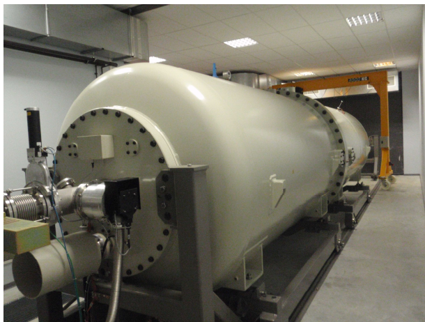
Fig. 35: AIFIRA facility. On the left, the 3.5 MV singletron; on the right the target chamber of the micrometric beamline.
