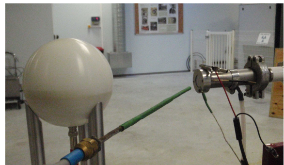
Fig. 58: On the left-side, response function of the 4.9" IRSN Bonner sphere (Se09); in red, energy range of the neutrons to be detected in this experiment. On the right-side, experimental setup for fluence measurements: Bonner sphere mounted on its base (left), end of the beam line with target, magnet and cable for current measurement (right), and target-cooling system (green).
