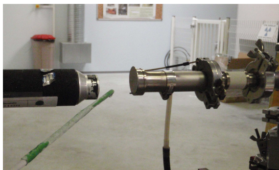
Fig. 59: Experimental setup for gamma measurements: on the left, end of the BGO spectrometer; on the right end of the beam line and target; in green, tube for air-cooling.
