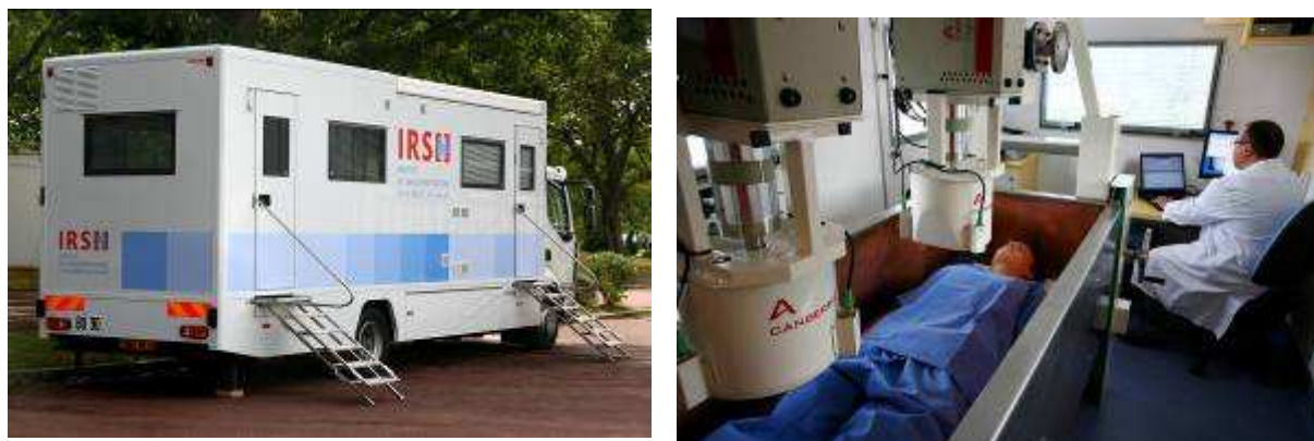
Figure 6.1. Photos of the IRSN LMA in vivo mobile unit and of the two installed germanium detectors.
