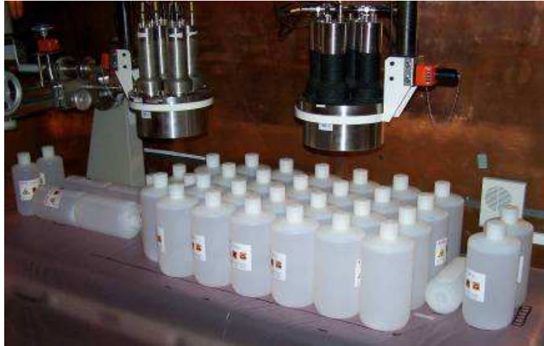
Figure 1.4. The SCHMIER bottle phantom used for whole body calibrations representing a 90 kg adult male subject.
