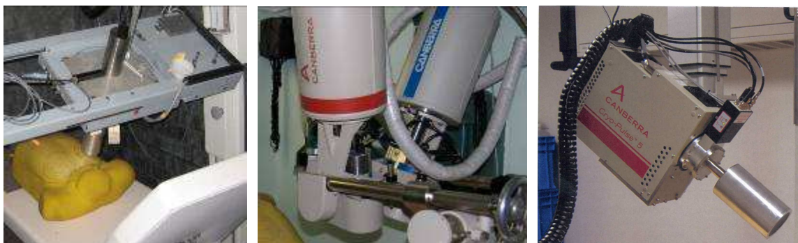
Figure 5.3. Photos of the three different germanium counting systems used for this study: IRSN's LOAX (left), CIEMAT's 4-LEGe (middle) and KIT's HPGe (right).
