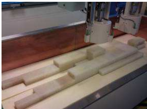
Figure 1.5. The IGOR bricks used for whole body calibrations of a typical counting system (left); Different configurations of the IGOR bricks representing respectively a 70 kg, 24 kg and 12 kg subject (right).
