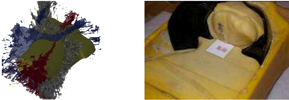
Figure 5.9. Positioning of the point perturbation source operated at KIT. Left: simulated tracks to determine the position for which there is an equal contribution of each organ; Right: positioning within the Livermore phantom.
