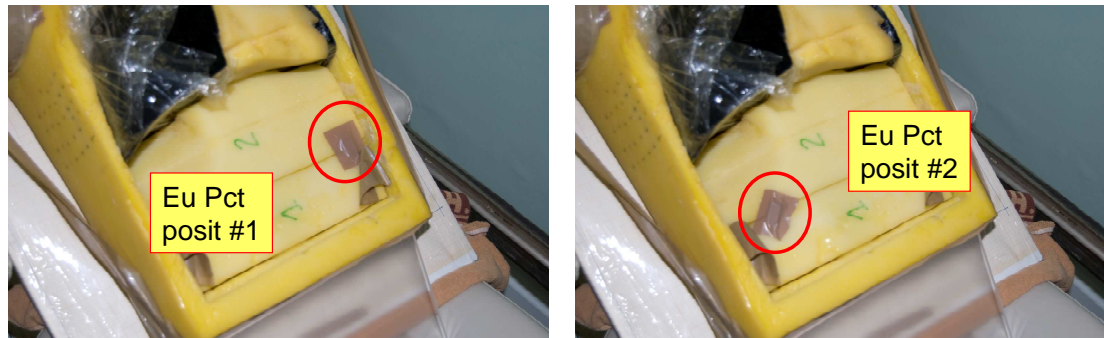
Figure 5.7. Operated positioning of the ^{152}\text{Eu} point source on the left and right side of the phantom at the level of the liver.
