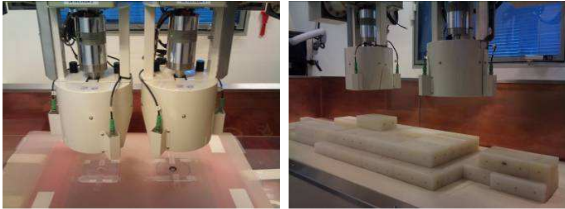
Figure 6.2. Visualization of the experimental measurements done with point sources (left) and with the IGOR phantom (right).
