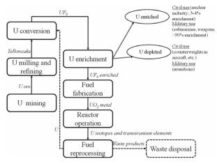
Figure 2. A simplified schema of the nuclear fuel cycle. Italicized words represent the forms of uranium at each stage of processing. Two end-products of uranium enrichment (enriched and depleted uranium) are presented. Dotted lines represent the additional stages of uranium processing.
