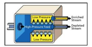
Figure 9. Gaseous diffusion technology. Source: Yale Scientific, assessed from http://www.yalescientific.org/2012/12/enriching-uranium/ [17 June 2015]
