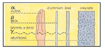
Figure 2. Penetration activity of the four main types of ionizing radiation. Source: World Nuclear Association, accessed from http://www.world-nuclear.org/info/Safetyand-Security/Radiation-and-Health/Radiation-and-Life/ [26 May 2015]
