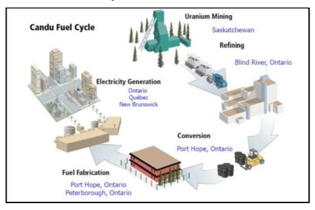
Figure 8. Canadian Candu nuclear fuel cycle. Source: Canadian Nuclear Waste Management Organization, assessed from http://www.nwmo.ca/uploads\_managed/MediaFiles/1162\_nwmo-nuclearfuelcycleandusedfu.pdf [19 June 2015].
