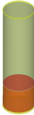
Figure 5.5: Mass-Geometry criticality system, depending on three parameters: radius, mass and concentration of fissile mass (in orange), inside a cylindrical container.
