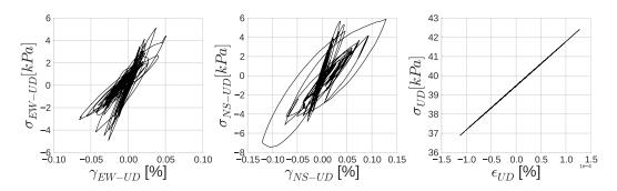
Fig. 3.6 Stress-strain curves on EW-UD component (left), NS-UD component (middle) and UD component (right) for point at GL-2.9 m of the WRLA.
