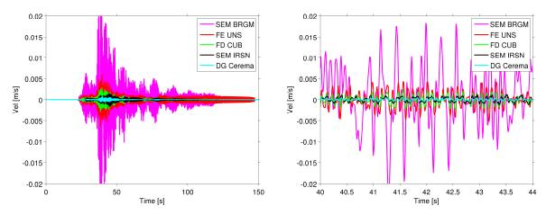
Figure 6: (left) Velocity seismograms at the top of the soil layer for the HF input signal. Reference solution in pink and differences of the other solutions to the reference. (right) Zoom from t=40 s to t=44 s.
