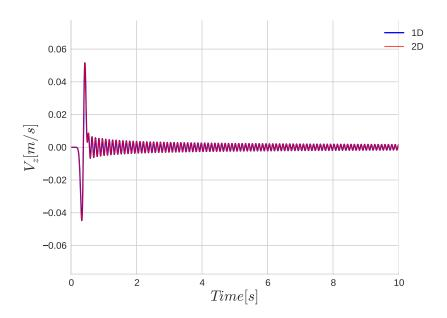
Fig. 4.39 Comparison of velocity outputs on z direction for 1D (in blue) and 2D (in red) SEM codes for pressure-dependent nonlinear P1 model with water table at midlayer under biaxial loading.
