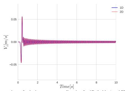
Fig. 4.36 Comparison of velocity outputs on z direction for 1D (in blue) and 2D (in red) SEM codes for pressure-dependent nonlinear P1 model with water table at surface level under biaxial loading.
