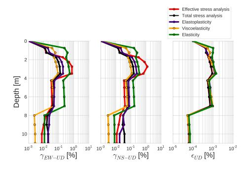
Fig. 3.42 Maximum strain profile of elastic (in green), viscoelastic (in orange), elastoplastic (in purple), visco-elastoplastic with no excess pore pressure development (in blue) and visco-elastoplastic with excess pore pressure development (in red) models for three components of Kushiro Port site.
