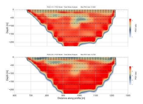
Fig. 5.24 Peak ground velocity ratio of the basin for total stress analysis on horizontal component for P-SV models of the 2D sedimentary basin model under loading of impulse source with PGA 0.05g (top), PGA 0.10g (middle) and 0.25g (bottom).
