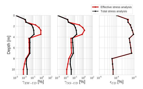
Fig. 3.40 Comparison of maximum strain profiles as a function of depth between viscoelastoplastic simulations with excess pore pressure development (in red) and without excess pore pressure development (in black) for EW-UD (left) and NS-UD (right) components.
