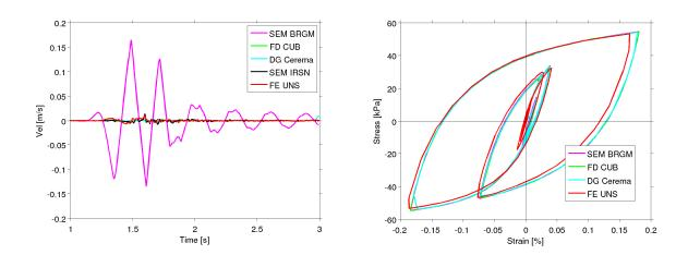
Figure 3: (Left) Velocity seismograms on the top of the soil layer (Z=0 m). The reference solution with hyperbolic non-linear model in pink. Differences to the reference for each team/code in other colors. (Right) Stress-strain curves near the middle of the layer (Z=13 m), Iwan model with 50 elasto-plastic elements at each node.
