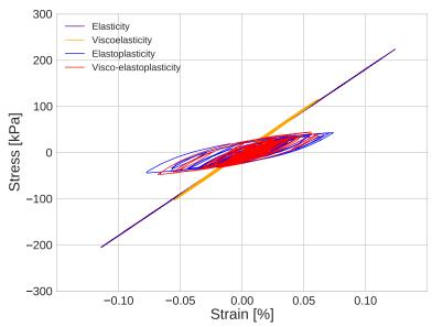
Fig. 2.19 Stress-strain curves for elasticity (in purple), viscoelasticity (in yellow), elastoplasticity (in blue) and visco-elastoplasticity (in red) for simulations under Real source #3 signal in the P1 model.
