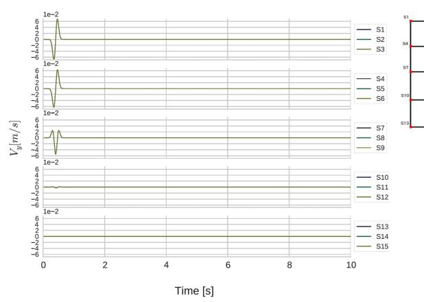
Fig. 4.20 Horizontal velocity outputs for all the stations of SH wave propagation model with two-element C-PML model.
