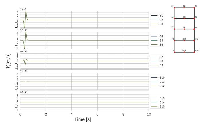
Fig. 4.18 Vertical velocity outputs for all the stations of P-SV wave propagation model with two-element C-PML model.
