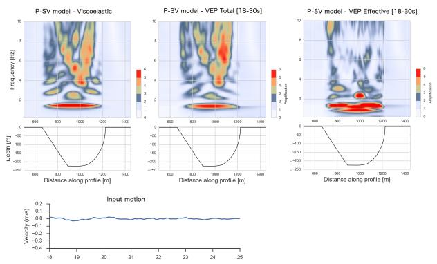
Fig. 5.35 Tranfer function of the second interval [18-30] s of P-SV model for viscoelasticity (at left), total stress analysis (at middle) and effective stress analysis (at right) under real input motion.
