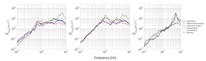
Fig. 3.26 Spectral acceleration comparison between elastic (in green), viscoelastic (in orange), elastoplastic (in purple), visco-elastoplastic with no excess pore pressure development (in blue) and visco-elastoplastic with excess pore pressure development (in red) models for three components of Kushiro Port site.
