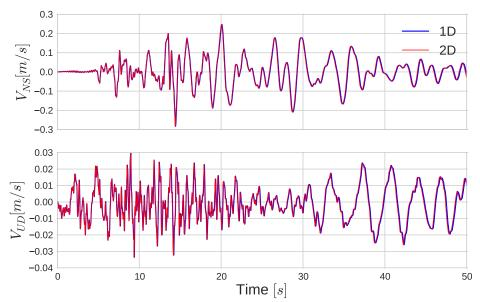
Fig. 4.47 Comparison of surface velocity outputs of WRLA model with single lateral element for NS (top) and for UD (bottom) directions between 1D (in blue) and 2D (in red) SEM codes.
