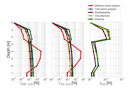
Fig. 3.13 Maximum strain profile of elastic (in green), viscoelastic (in orange), elastoplastic (in purple), visco-elastoplastic with no excess pore pressure development (in blue) and visco-elastoplastic with excess pore pressure development (in red) models for three components.
