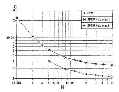
Fig. 2.22 Values for the minimum number of points per wavelength (G) versus the polynomial order (N) for FEM and SEM, at a distance of 960 grid points. Estimations of G were done, taking into account the mean value of element size (dx mean) (solid line) and the maximum element size (dx max) (dashed line) (after Seriani and Priolo 1991[144]; 1993 [127]).
