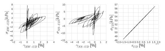
Fig. 3.7 Stress-strain curves on EW-UD component (left), NS-UD component (middle) and UD component (right) for point at GL-4.0 m of the WRLA.
