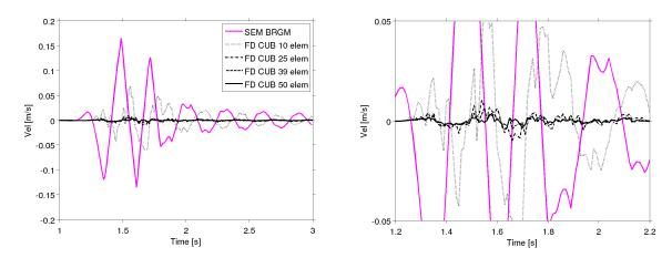
Figure 4: (Left) Velocity seismograms at the top of the soil layer. Reference solution in pink and different solutions for CUB team with different number of Iwan elements per node. (Right) zoom of the previous figure to better appreciate differences between results using increasing number of elements.
