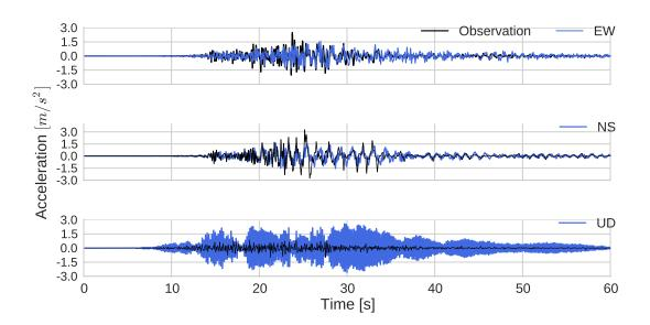
Fig. 3.23 Surface acceleration time histories on three directions for the simulation without pore pressure effects (in blue) and observation (in black) at the KP.
