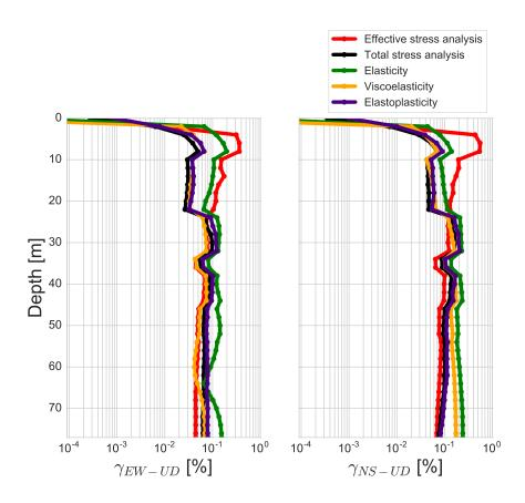
Fig. 3.27 Maximum strain profile of elastic (in green), viscoelastic (in orange), elastoplastic (in purple), visco-elastoplastic with no excess pore pressure development (in blue) and visco-elastoplastic with excess pore pressure development (in red) models for three components of Kushiro Port site.
