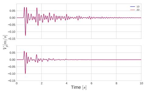
Fig. 4.45 Comparison of velocity outputs of Volvi model with single-element C-PML for elasticity (top) and for viscoelasticity (bottom) between 1D (in blue) and 2D (in red) SEM codes.
