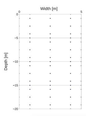
Fig. 4.1 Two-dimensional mesh used in 2D SEM code for P1 model, shown with GLL point distribution. Solid lines hold for elementary boundaries.
