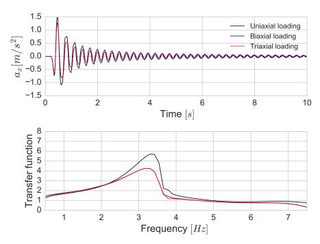
Fig. 3.2 Surface acceleration time histories (top); Fourier amplitudes of surface acceleration for uniaxial loading (in black), biaxial loading (blue) and triaxial loading (in red) for P1 model (bottom).
