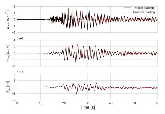
Fig. 3.28 Surface acceleration (top), velocity (middle) and displacement (bottom) comparison between uniaxial (in black) and triaxial (in red) loading for NS component.
