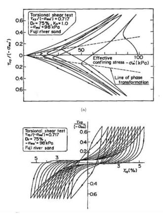
Fig. 1.11 Stress path (top) and stress-strain diagram (bottom) for dense sand after experimental results (after Ishihara, 1985 [74]).
