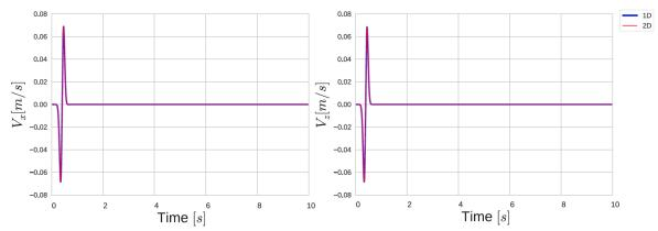
Fig. 4.24 Comparison of velocity outputs on horizontal (left) and vertical (right) directions of P-SV wave propagation model with upward attenuation C-PML element between 1D (in blue) and 2D (in red) SEM codes.
