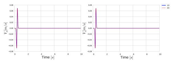
Fig. 4.14 Comparison of velocity outputs on horizontal (left) and vertical (right) directions of P-SV wave propagation model with single-element C-PML between 1D (in blue) and 2D (in red) SEM codes.
