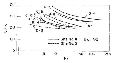
Fig. 5.3 Liquefaction resistance curves for different soil samples in Kushiro Port site (after Iai et al. 1995 [71]).
