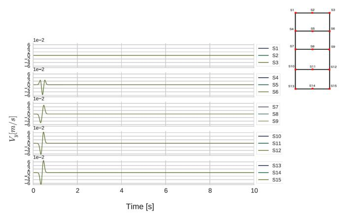
Fig. 4.25 Horizontal velocity outputs for all the stations of SH wave propagation model with upward attenuation C-PML element.
