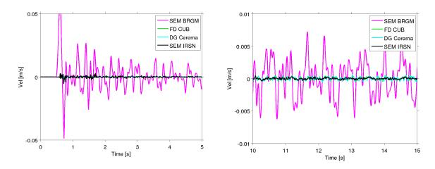
Figure 9: Velocity seismograms at the surface. Volvi soil column: velocity seismogram at Z=0 m of BRGM team in pink and differences to all other teams in other colors (left) between 0 and 5 seconds and (right) between 10 and 15 seconds (different vertical axis).
