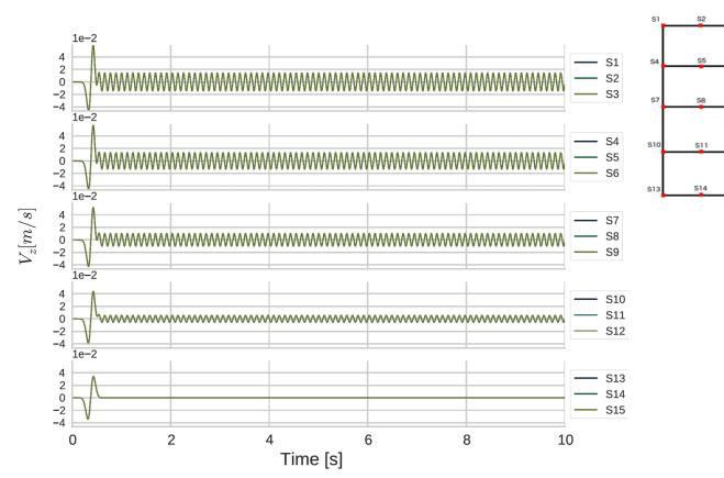
Fig. 4.3 Vertical velocity outputs for all the stations of P-SV wave propagation model with borehole condition.
