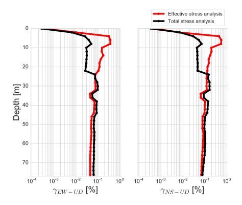
Fig. 3.25 Comparison of maximum strain profiles as a function of depth between viscoelastoplastic simulations with excess pore pressure development (in red) and without excess pore pressure development (in black) for EW-UD (left) and NS-UD (right) components.
