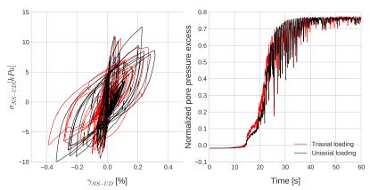
Fig. 3.29 (a) Stress-strain curve comparison between uniaxial (in black) and triaxial (in red) loading results for NS-UD component at GL-4 m, (b) Excess pore pressure vs time comparison between uniaxial (in black) and triaxial (in red) loading results at GL-4 m.
