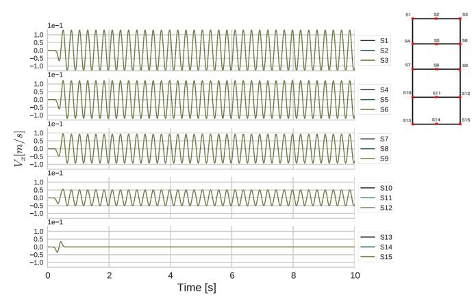
Fig. 4.2 Horizontal velocity outputs for all the stations of P-SV wave propagation model with borehole condition.
