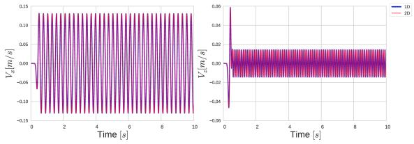
Fig. 4.4 Comparison of velocity outputs on horizontal (left) and vertical (right) directions of P-SV wave propagation model with borehole condition between 1D (in blue) and 2D (in red) SEM codes.
