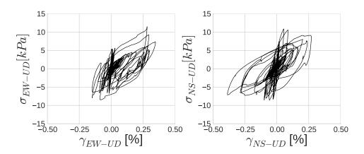
Fig. 3.21 Stress-strain curves on EW-UD component (left) and NS-UD component (right) for point at GL-4 m of the KP.
