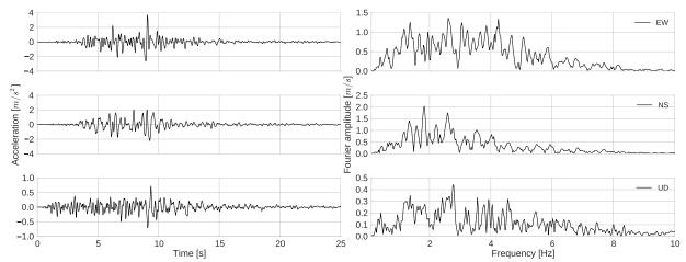
Fig. 5.11 Acceleration time histories (left column) and Fourier amplitudes (right column) of Northridge earthquake records for EW component (top), NS component (middle) and vertical component (bottom).
