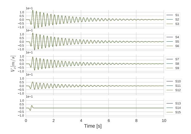
Fig. 4.27 Horizontal velocity outputs for all the stations of P-SV wave propagation model with viscoelastic rheology in P1 medium.
