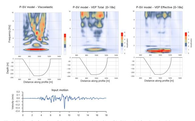
Fig. 5.34 Tranfer function of the initial interval [0-18] s of P-SV model for viscoelasticity (at left), total stress analysis (at middle) and effective stress analysis (at right) under real input motion.
