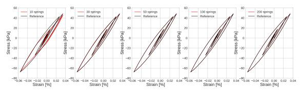
Fig. 2.27 Stress-strain curves for all the models with reference model solution (in black).
