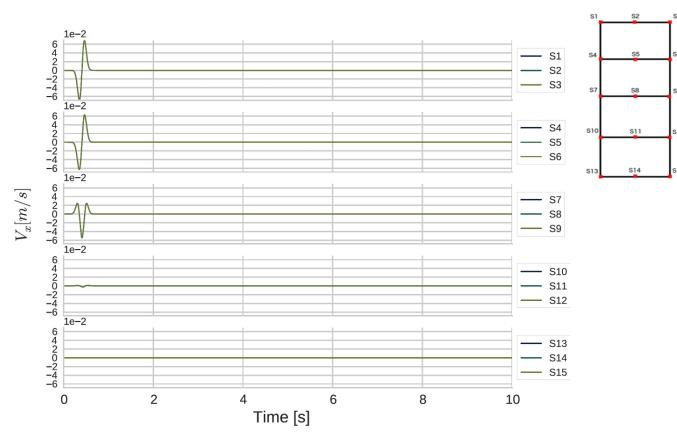
Fig. 4.17 Horizontal velocity outputs for all the stations of P-SV wave propagation model with two-element C-PML model.
