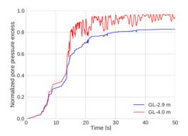
Fig. 3.8 Recorded pore pressure change at GL-2.9 m of the WRLA (left) (extracted from Holzer and Youd, 2007 [67] and modified after Pham, 2013); Pore pressure excess temporal change for the point at GL-2.9 m (in blue) and for the point at GL-4.0 m (in red) of the WRLA (right).
