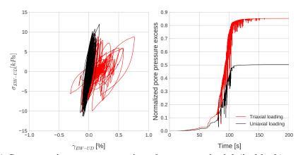
Fig. 3.45 (a) Stress-strain curve comparison between uniaxial (in black) and triaxial (in red) loading results for EW-UD component at GL-2.75 m, (b) Excess pore pressure vs time comparison between uniaxial (in black) and triaxial (in red) loading results at GL-2.75 m.
