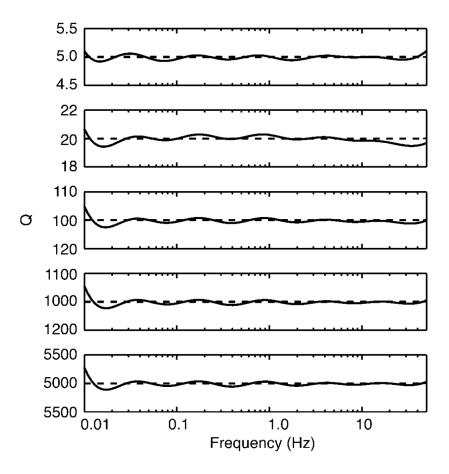
Fig. 1.5 The fit between model Q and target Q value of 5 (top panel), 20 (second panel), 100 (third panel), 1000 (fourth column) and 5000 (bottom panel) in frequency band of 0.01 - 50Hz (after Liu and Archuleta, 2006 [98]).
