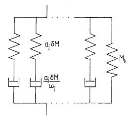
Fig. 1.4 Rheological model for generalized Maxwell body with viscosities  $a_j \frac{\delta M}{\omega_j}$  and elastic moduli  $a_j \delta M$  (after Emmerich and Korn, 1987 [40]).
