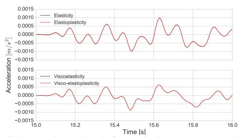
Fig. 2.17 Acceleration time histories for elasticity (in black) and elastoplasticity (in red) (top); Acceleration time histories for viscoelasticity (in black) and visco-elastoplasticity (in red) (bottom) on [15-16] s time interval for simulations under Real source #3 signal in the P1 model.
