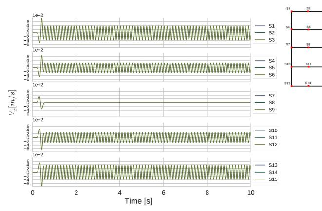
Fig. 4.7 Horizontal velocity outputs for all the stations of P-SV wave propagation model with incident wave field.
