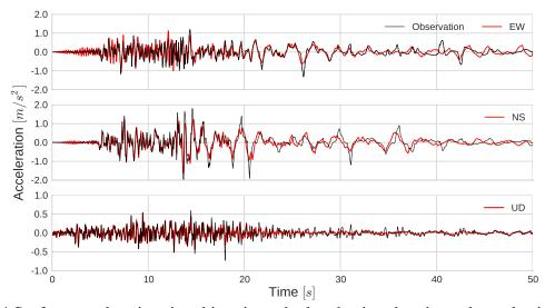
Fig. 3.4 Surface acceleration time histories calculated using the visco-elastoplastic model with pore pressure effects (in red) and real records (in black) for the WRLA site.
