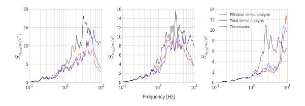
Fig. 3.39 Acceleration spectra of recorded surface acceleration (in black), visco-elastoplastic SEM simulation with excess pore pressure development (in red) and without excess pore pressure development (in blue) for EW component (left); for NS component (right)
