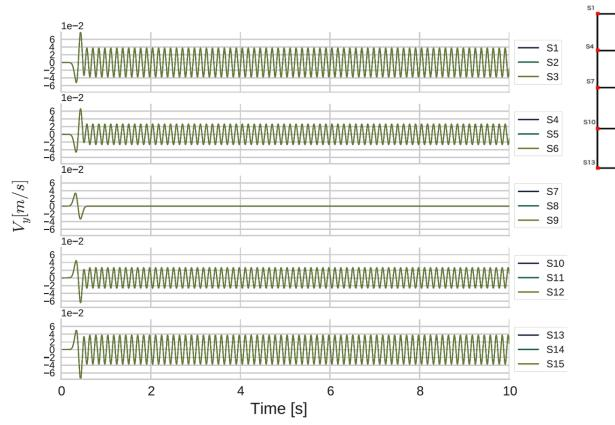
Fig. 4.10 Horizontal velocity outputs for all the stations of SH wave propagation model with incident wave field.
