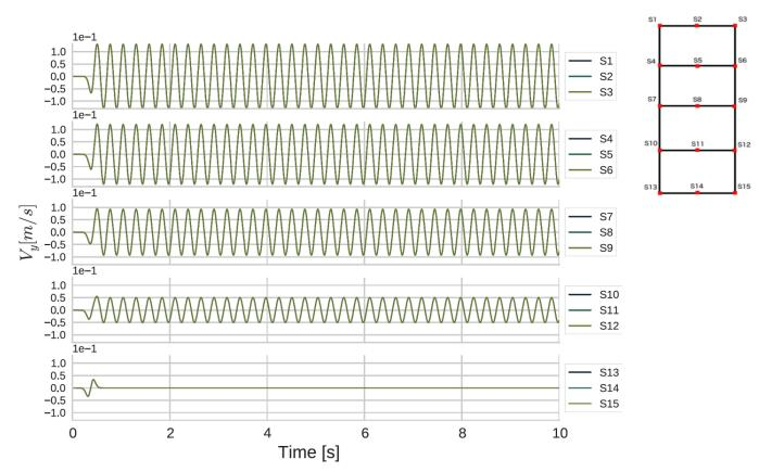
Fig. 4.5 Horizontal velocity outputs for all the stations of SH wave propagation model with borehole condition.
