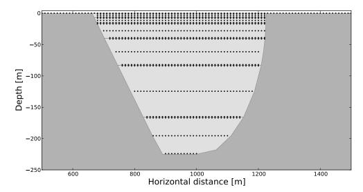
Fig. 5.8 Velocity receivers located on the 2D model.
