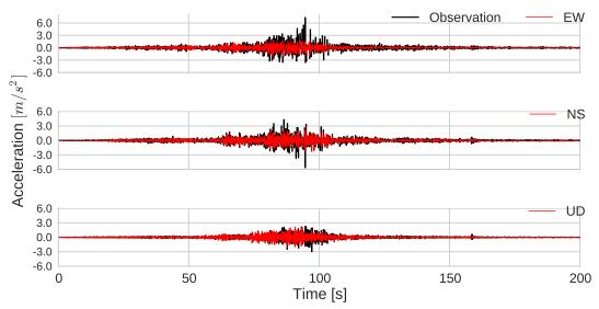
Fig. 3.32 Output acceleration time histories calculated in visco-elastoplastic model with excess pore pressure generation (in red) and real records (in black) of OP.
