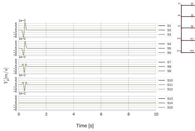
Fig. 4.15 Horizontal velocity outputs for all the stations of SH wave propagation model with single-element C-PML model.
