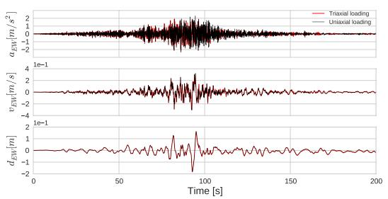
Fig. 3.43 Surface acceleration (top), velocity (middle) and displacement (bottom) comparison between uniaxial (in black) and triaxial (in red) loading for EW component.
