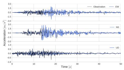
Fig. 3.9 Surface acceleration time histories on three directions for the simulation without pore pressure effects (in blue) and observation (in black) at the WRLA.
