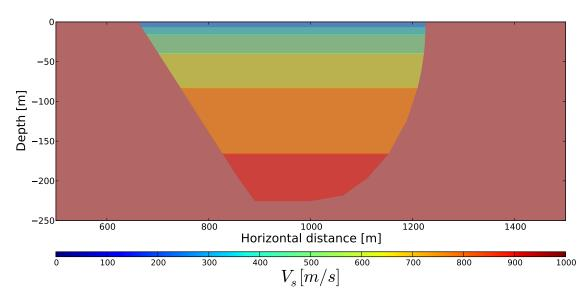
Fig. 5.1 Shear wave velocity profile of the 2D sedimentary basin model where bedrock shear velocity is 2000 m/s.
