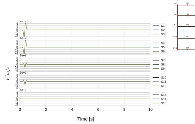
Fig. 4.13 Vertical velocity outputs for all the stations of P-SV wave propagation model with single-element C-PML model.
