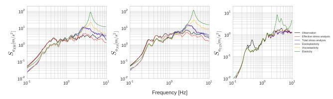
Fig. 3.12 Spectral acceleration comparison between elastic (in green), viscoelastic (in orange), elastoplastic (in purple), visco-elastoplastic with no excess pore pressure development (in blue) and visco-elastoplastic with excess pore pressure development (in red) models for three components.
