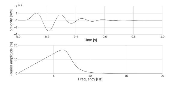
Fig. 2.4 Velocity time histories (left); Fourier amplitude (right) of the input motion used in Rome model.
