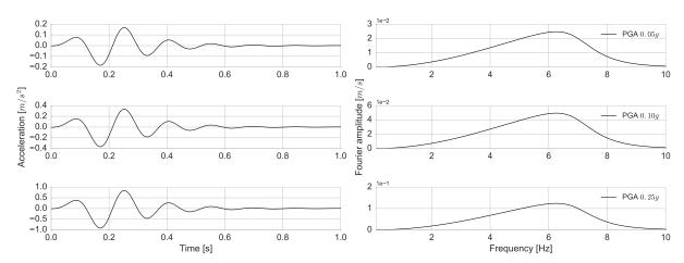
Fig. 5.10 Acceleration time histories (left column) and Fourier amplitudes (right column) of impulse sources with PGA 0.05g (top), PGA 0.10g (middle) and PGA 0.25g (bottom).
