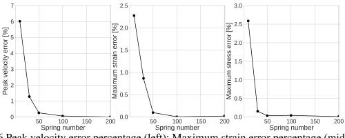
Fig. 2.26 Peak velocity error percentage (left); Maximum strain error percentage (middle); Maximum stress error (right) for the solutions of all the models.
