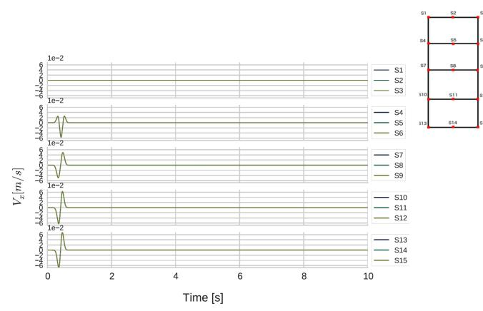
Fig. 4.22 Horizontal velocity outputs for all the stations of P-SV wave propagation model with upward attenuation C-PML element.
