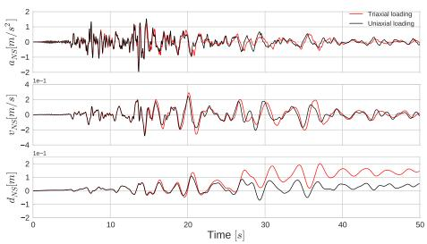
Fig. 3.14 Surface acceleration (top), velocity (middle) and displacement (bottom) comparison between uniaxial (in black) and triaxial (in red) loading for NS component.
