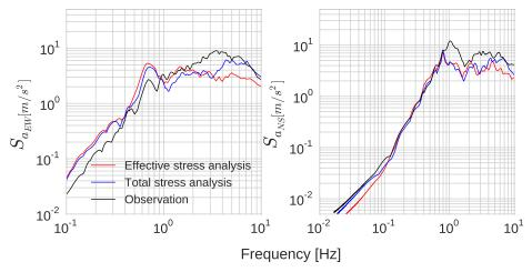
Fig. 3.24 Acceleration spectra of recorded surface acceleration (in black), visco-elastoplastic SEM simulation with excess pore pressure development (in red) and without excess pore pressure development (in blue) for EW component (left); for NS component (right)
