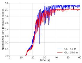
Fig. 3.19 Pore pressure excess temporal change for the point at GL-4.0 m (in blue) and for the point at GL-15.0 m (in red) of the KP.
