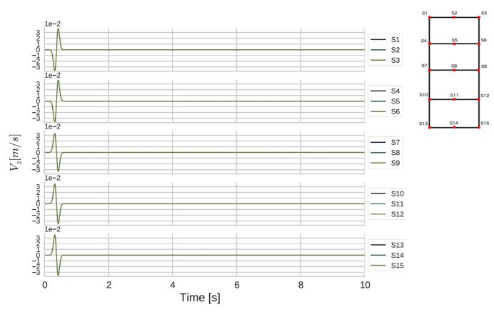
Fig. 4.8 Vertical velocity outputs for all the stations of P-SV wave propagation model with incident wave field.
