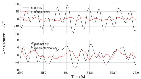
Fig. 2.18 Acceleration time histories for elasticity (in black) and elastoplasticity (in red) (top); Acceleration time histories for viscoelasticity (in black) and visco-elastoplasticity (in red) (bottom) on [35-36] s time interval for simulations under Real source #3 signal in the P1 model.
