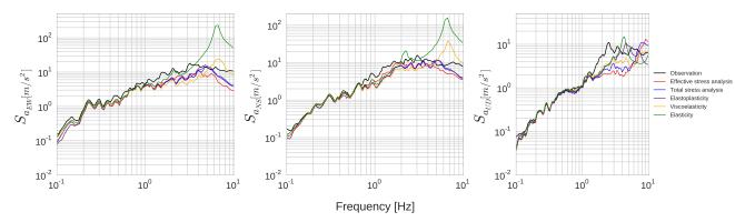
Fig. 3.41 Spectral acceleration comparison between elastic (in green), viscoelastic (in orange), elastoplastic (in purple), visco-elastoplastic with no excess pore pressure development (in blue) and visco-elastoplastic with excess pore pressure development (in red) models for three components of Kushiro Port site.
