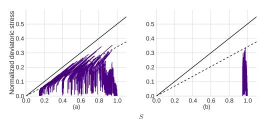
Fig. 3.35 (a) Deviatoric plan for point at GL-2.75 m, (b) Deviatoric plan for point at GL-5 m of the OP model with failure line (solid line) and phase transformation line (dashed line).
