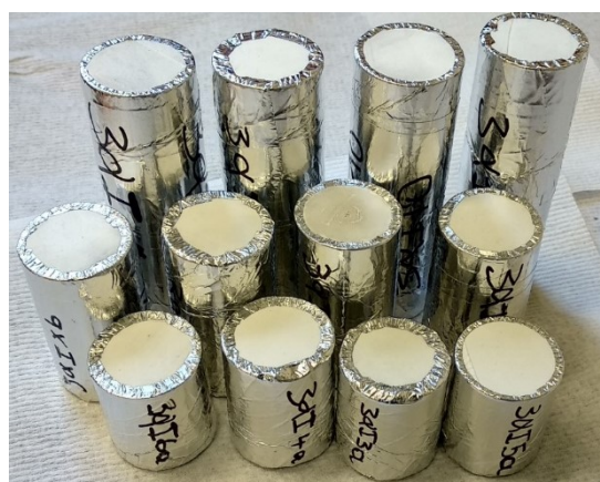
Figure 10: Pastes covered with adhesive aluminium foil after conditioning and prior to carbonation.
