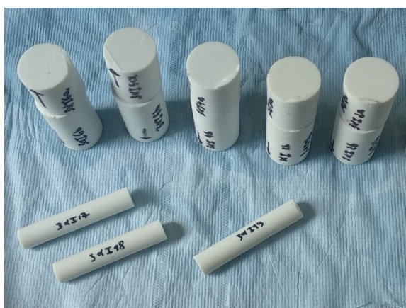
Figure 9: Fabricated pastes C/S = 3 : shrinkage samples ( \varnothing = 14 mm H = 90 mm) and remaining samples ( \varnothing = 30 mm H = 120 mm) cut to generate samples of different lengths for different carbonation terms.
