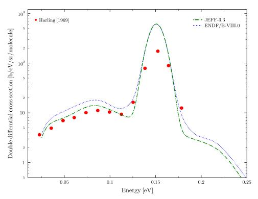
FIGURE 3.17: Double differential scattering cross section of light water at incident energy E=151~meV and scattering angle  $\theta$ =15°.
