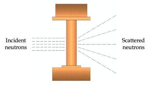
FIGURE 4.5: Schematics of the TOF measurements.
