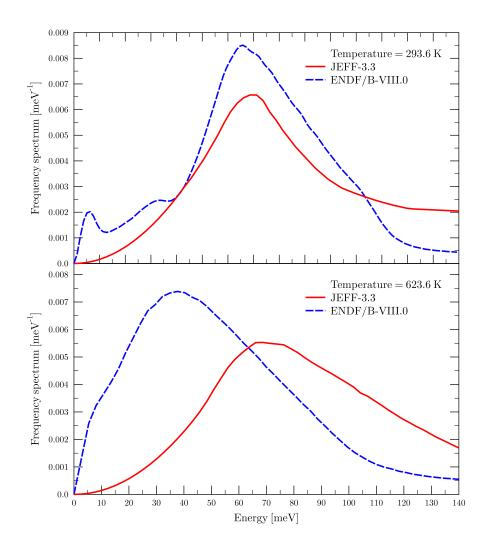
FIGURE 3.10: Frequency spectrum of light water based on the JEFF-3.3 and ENDF/B-VIII.0 at 293.6 K (top) and 623.6 K (bottom).
