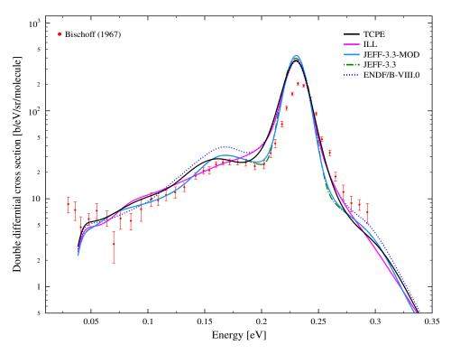
FIGURE 7.4: Double differential scattering cross section of light water at incident energy E=231~meV and scattering angle  $\theta$ =25°.
