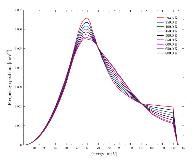
FIGURE 3.5: Frequency spectrum of light water based on ENDF/B-VII.1 TSL evaluation.
