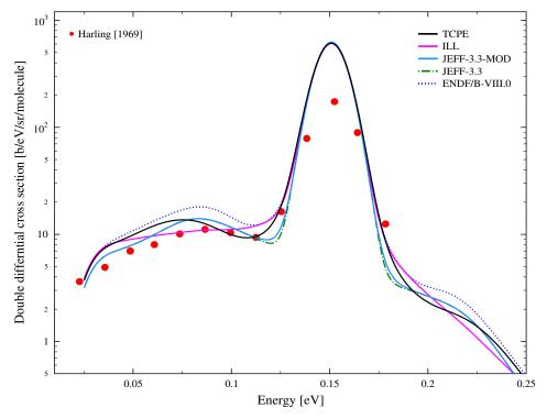
FIGURE 7.5: Double differential scattering cross section of light water at incident energy E=151~meV and scattering angle  $\theta$ =15°.
