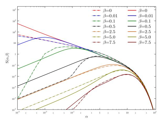
FIGURE 3.12:  $S(\alpha, \beta)$  at 573.6 K as a function of  $\alpha$  for different  $\beta$  values. The solid lines represent the ENDF/B-VIII.0 TSL evaluation whereas the dotted lines represent the JEFF-3.3 TSL evaluation for light water.
