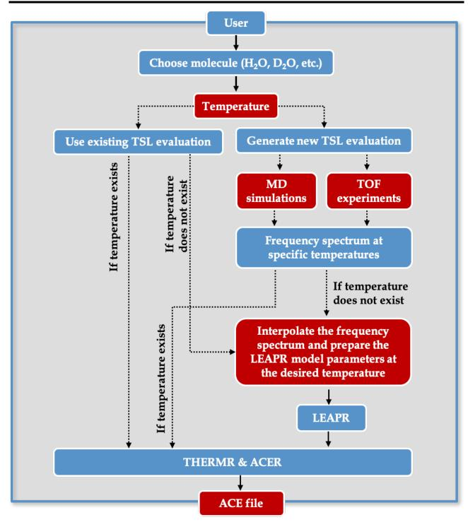
FIGURE 6.2: Block diagram of the SAB module of the GAIA 2 code.
