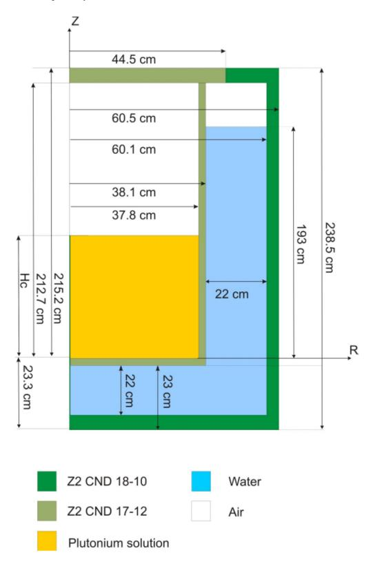
FIGURE 6.4: Benchmark model for the plutonium nitrate temperature effect experimental program [65].
