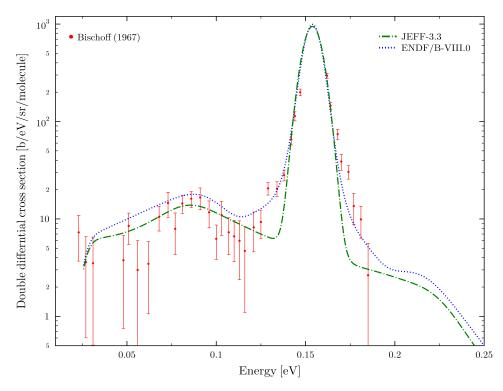
FIGURE 3.13: Double differential scattering cross section of light water at incident energy E=154~meV and scattering angle  $\theta$ =14°.
