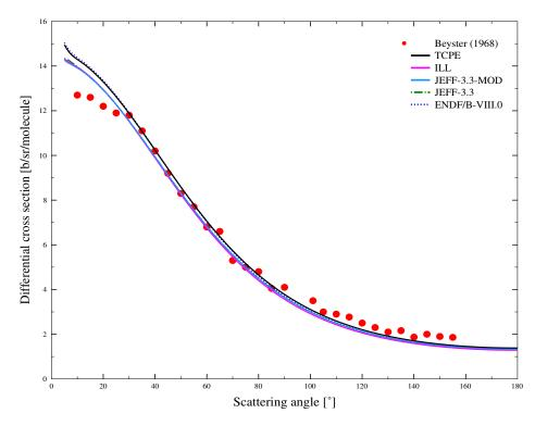
FIGURE 7.10: Differential cross section for light water at  $E=179~\mathrm{meV}$ .
