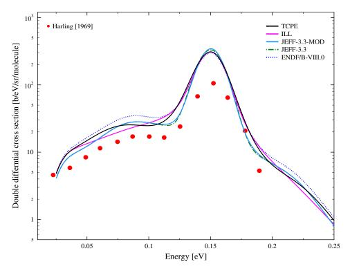
FIGURE 7.6: Double differential scattering cross section of light water at incident energy E=151~meV and scattering angle  $\theta$ =32°.
