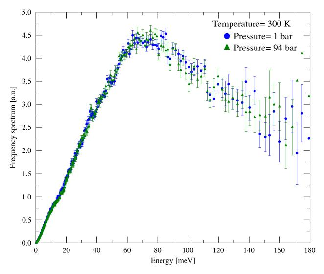
FIGURE 4.22: Frequency spectrum of light water measured at the IN4c for different pressures at 300 K.
