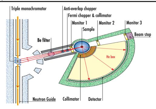
FIGURE 4.7: Experimental setup of the IN6 TOF spectrometer.
