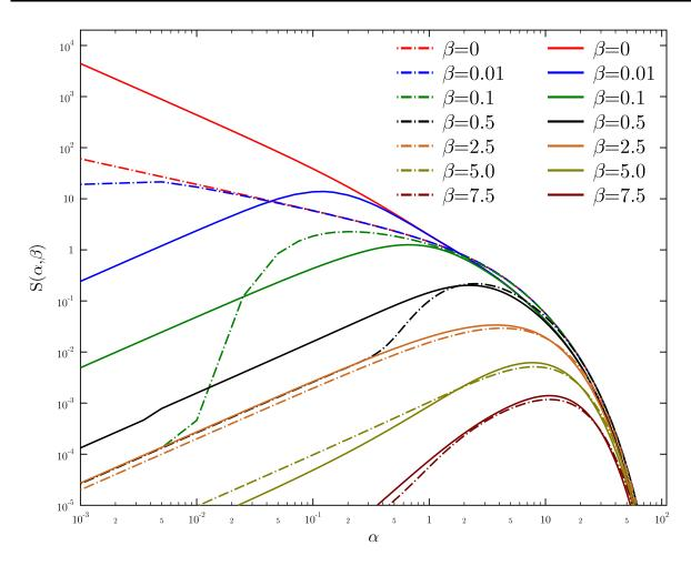
FIGURE 3.11:  $S(\alpha, \beta)$  at 293.6 K as a function of  $\alpha$  for different  $\beta$  values. The solid lines represent the ENDF/B-VIII.0 TSL evaluation whereas the dotted lines represent the JEFF-3.3 TSL evaluation for light water.
