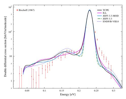
FIGURE 7.3: Double differential scattering cross section of light water at incident energy E=231~meV and scattering angle  $\theta$ =14°.
