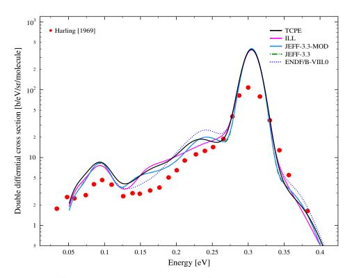
FIGURE 7.7: Double differential scattering cross section of light water at incident energy E=305~meV and scattering angle  $\theta$ =15°.
