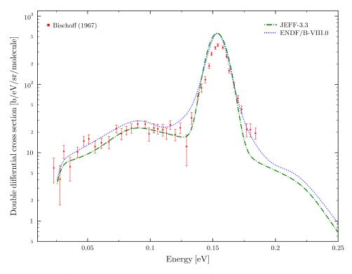
FIGURE 3.14: Double differential scattering cross section of light water at incident energy E=154~meV and scattering angle  $\theta$ =25°.
