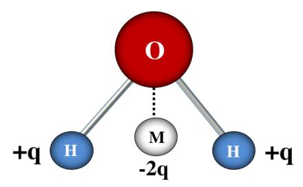
FIGURE 5.1: TIP4P/2005f water model.
