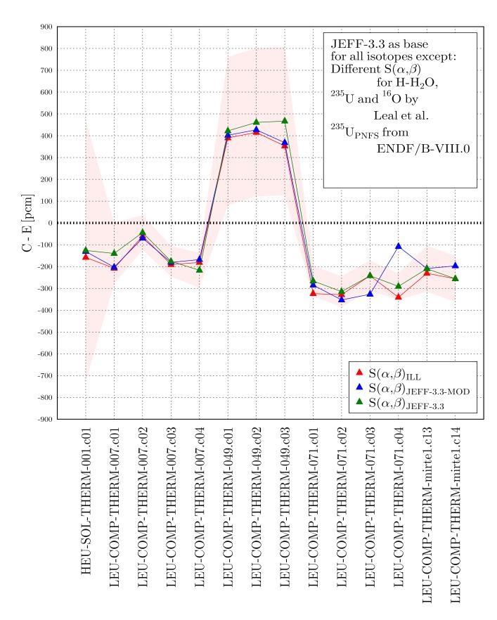
FIGURE 7.15: Calculated - Experimental (C-E) results for the selected ICSBEP benchmark using different TSL evaluations, new IRSN  $^{16}$ O and  $^{235}$ U evaluations. In addition, the new  $^{235}$ U prompt fission neutron cross section from ENDF/B-VIII.0 has been used in this study.
