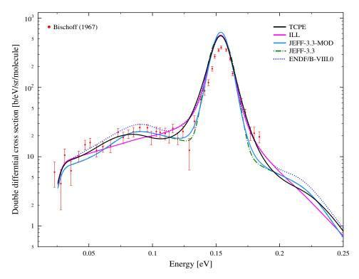
FIGURE 7.2: Double differential scattering cross section of light water at incident energy  $E=154~{\rm meV}$  and scattering angle  $\theta$ =25°.
