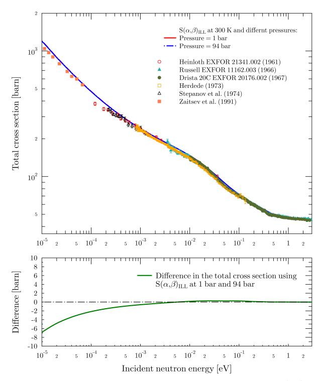
FIGURE 4.27: Comparison of the total cross section of light water at 300.0 K based on  $S(\alpha, \beta)_{ILL}$  at 1 bar and 94 bar, along with the EXFOR experimental data.
