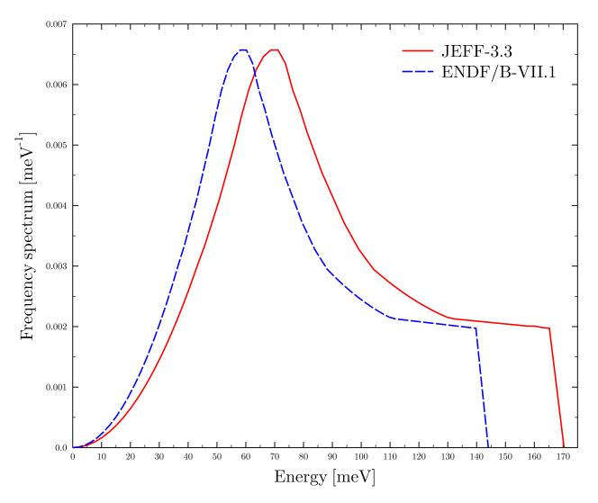
FIGURE 3.4: Frequency spectrum of light water based on the JEFF-3.3 and ENDF/B-VII.1 TSL evaluation.
