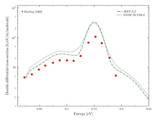
FIGURE 3.18: Double differential scattering cross section of light water at incident energy E=151~meV and scattering angle  $\theta$ =32°.
