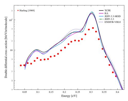
FIGURE 7.8: Double differential scattering cross section of light water at incident energy E=305~meV and scattering angle  $\theta$ =30°.
