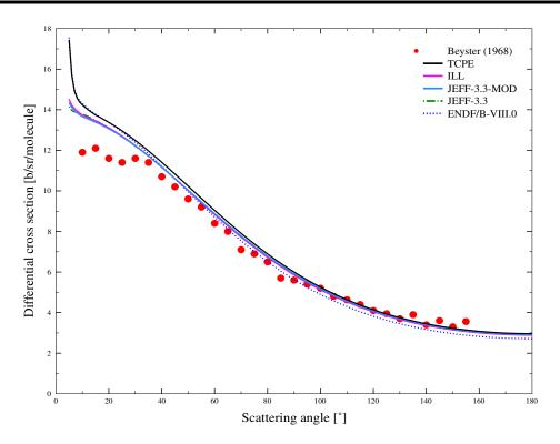
FIGURE 7.9: Differential cross section for light water at  $E=56.9~\mathrm{meV}$ .
