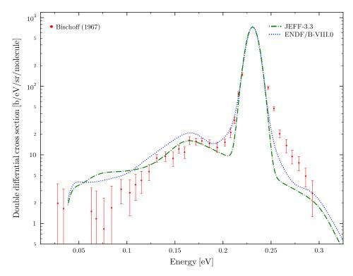
FIGURE 3.15: Double differential scattering cross section of light water at incident energy E=231~meV and scattering angle  $\theta$ =14°.
