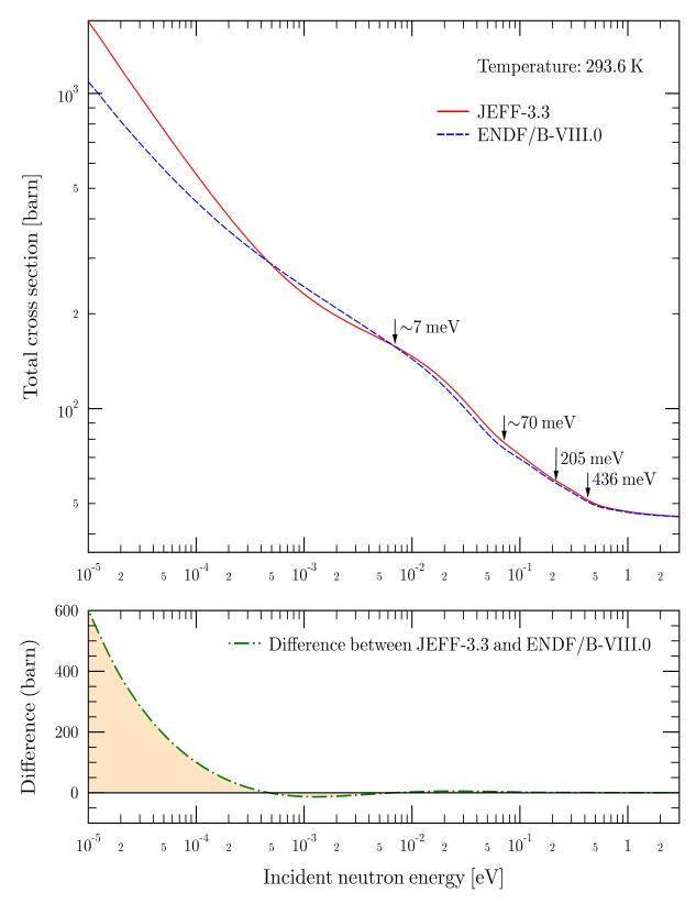
FIGURE 3.24: Comparison of the total cross section of light water at 293.6 K based on JEFF-3.3 and ENDF/B-VIII.0 TSL evaluations.
