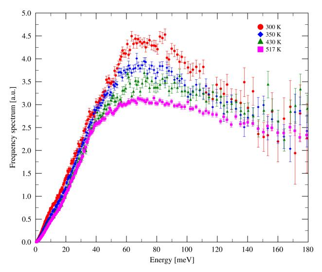
FIGURE 4.24: Frequency spectrum of light water measured at the IN4c at different temperatures.
