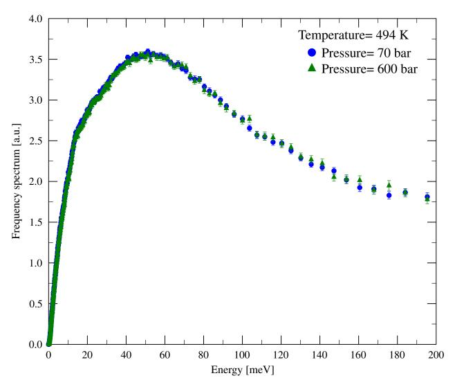
FIGURE 4.23: Frequency spectrum of light water measured at the IN6 at different pressures at 494 K.
