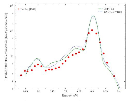
FIGURE 3.19: Double differential scattering cross section of light water at incident energy  $E=305~{\rm meV}$  and scattering angle  $\theta$ =15°.
