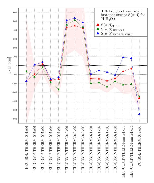
FIGURE 7.17: Calculated - Experimental (C-E) results for the selected ICSBEP benchmark using different TSL evaluations.
