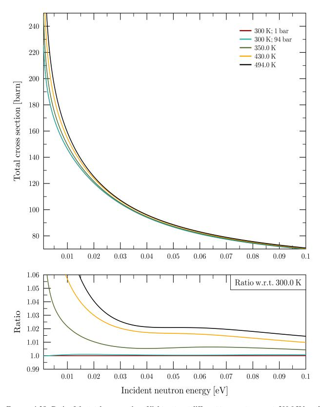
FIGURE 4.28: Ratio of the total cross section of light water at different temperatures w.r.t. 300.0 K based on  $S(\alpha,\beta)_{\rm ILL}$ .
