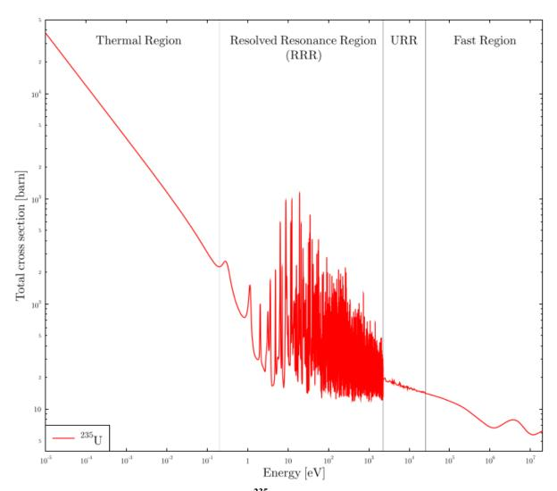
FIGURE 1.1: Total cross section of <sup>235</sup>U as a function of incident neutron energy.
