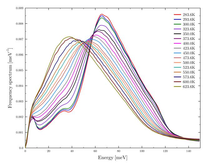
FIGURE 3.6: Frequency spectrum of light water based on the ENDF/B-VIII.0 TSL evaluation.
