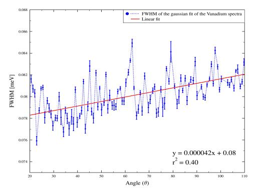
FIGURE 4.15: FWHM of the Gaussian fit of the Vanadium spectra obtained from the IN6.
