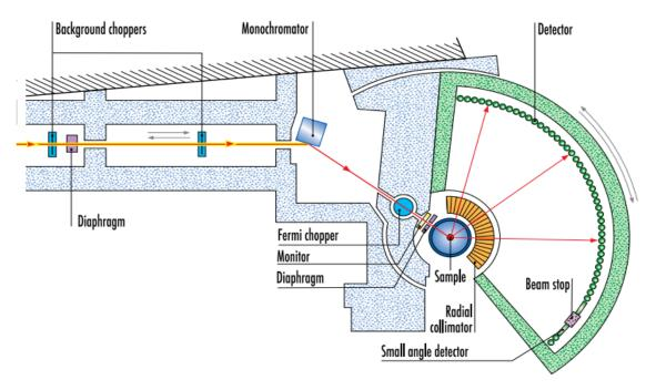
FIGURE 4.6: Experimental setup of the IN4c TOF spectrometer [46].
