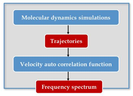
FIGURE 5.3: Block diagram of the MD data analysis.
