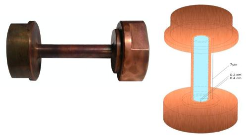
FIGURE 4.4: CuBe pressure cell (sample holder).
