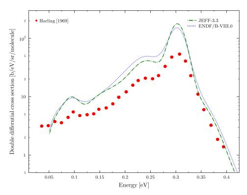
FIGURE 3.20: Double differential scattering cross section of light water at incident energy E=305 meV and scattering angle  $\theta$ =30°.
