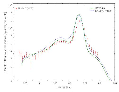
FIGURE 3.16: Double differential scattering cross section of light water at incident energy E=231~meV and scattering angle  $\theta$ =25°.
