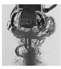
Figure 6.12: Snapshot of the discharge of a silo immersed in water with an instantaneous rupture of the outlet for L = 40mm, D = 10mm,  $d_p = 180 \mu m$  (hydrophobic ceramic particles) and  $h_{water} \approx 80$ mm.
