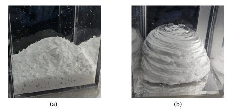
Figure 6.4: Comparison of the macroscopical behavior between (a) untreated and (b) hydrophobic ceramic particles, with  $d_p = 180 \mu m$ , poured in a water tank.
