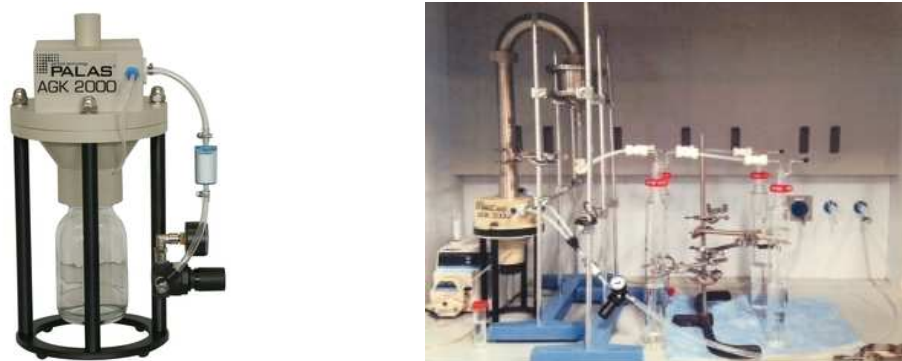
Figure 4-1 Aerosol deposition device PALAS AGK-2000 (left); and the experimental setup (right).
